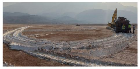
Salt tailings has little mass strength under no confining pressure (very low moisture contents ("dry")).
