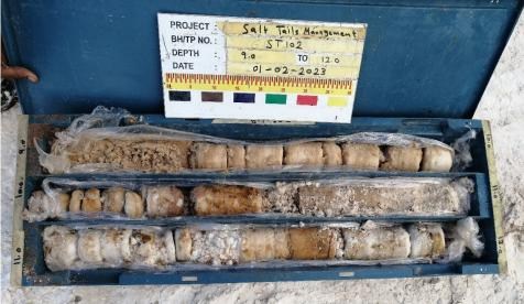
Fragmented disks of salt, or even pulverised material. Samples were highly disturbed during drilling (even when using double coring)
