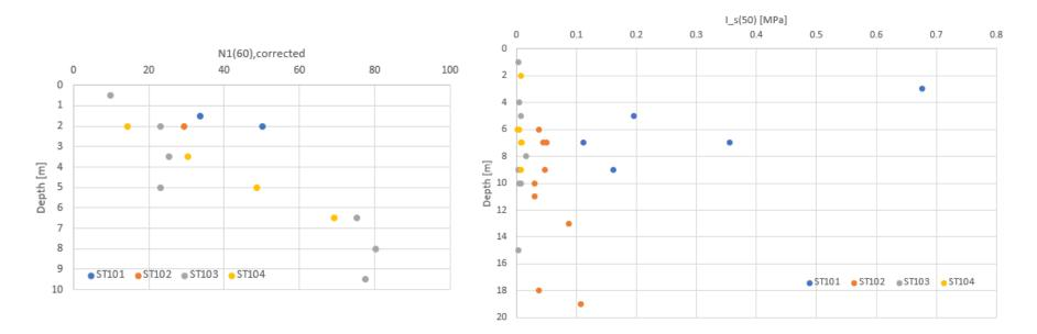
Clear relation to the disposal strategy. Boreholes ST103 and ST104 have lower strength both in-situ and in the laboratory.
