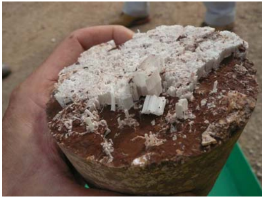
Gypsum needles crystal growth on open discontinuities
