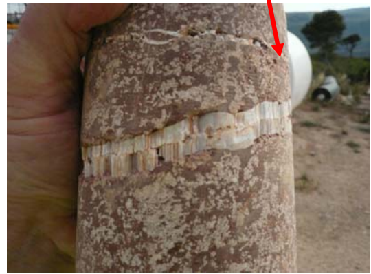
Gypsum needles crystal growth on open discontinuities
