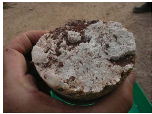
Gypsum needles crystal growth on open discontinuities
