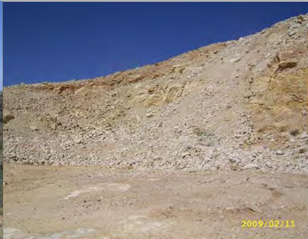
Inspection visit allowed assessment of armourstone quality and impression of the quantity of large rock blocks available. There were doubts if enough thick layers were available. The rock is locally brecciated, fractured and weathered.
