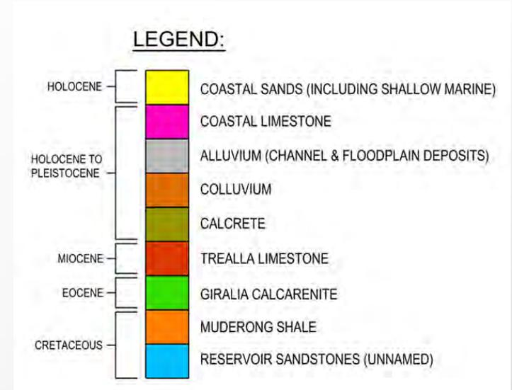
The island is shaped by an anticlinal fold structure, that also acts as a trap for the oil, which is arrested by the Muderong Shale, which underlies the Tertiary Limestone rock
