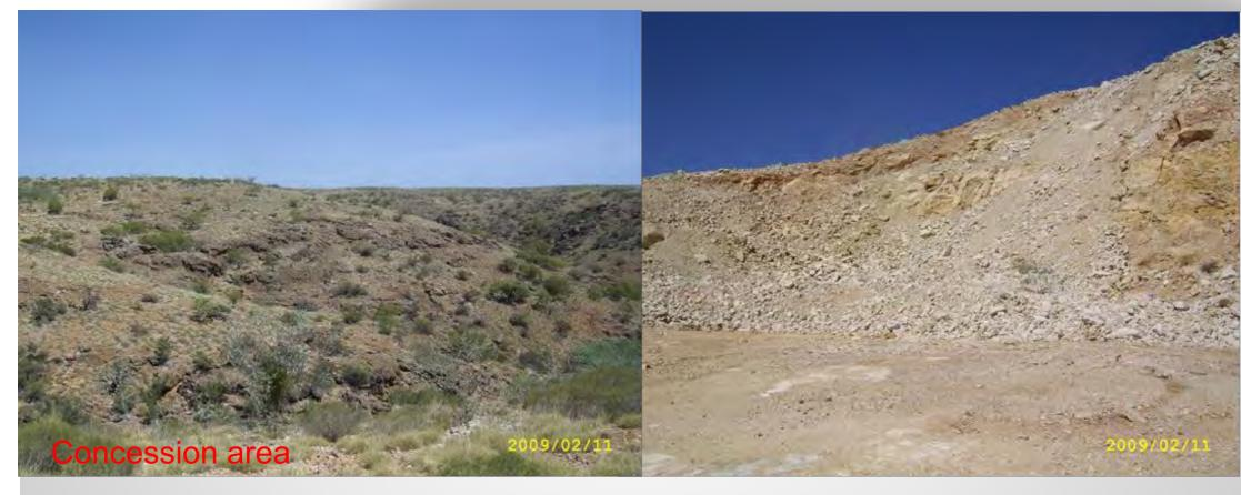
Inspection visit allowed assessment of armourstone quality and impression of the quantity of large rock blocks available. There were doubts if enough thick layers were available. The rock is locally brecciated, fractured and weathered.
