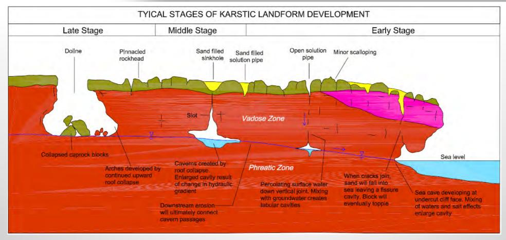
Weathering results in karst by dissolution. Rusty oxidation and clay weathering products occur. Also a duricrust (calcrete caprock) is developed.
