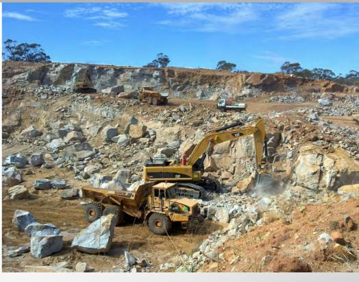
Rock was sourced with 4 different suppliers, multiple quarries. The way they achieved to produce a compliant end-product differed significantly based on geology, rock mass properties, blasting performance and rock selection methods.
