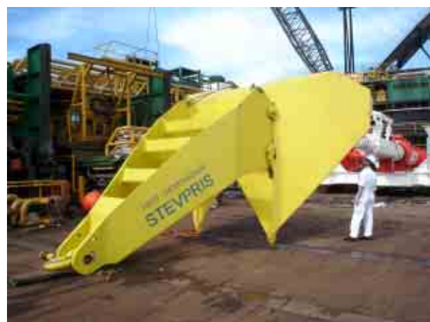
Figure 4 - Vryhof Stevpris New Generation drag anchor ready to be installed offshore Tuban, Indonesia.
