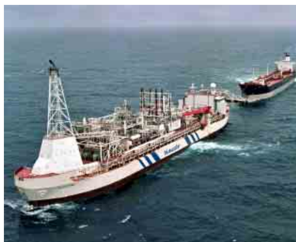
Figure 2 - The Bluewater FPSO "Glas Dour" offloading to a shuttle tanker.
