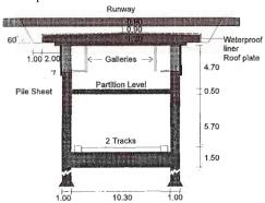
Figure 3 Undercutting beneath a Sub-terrain Roof Plate (all measures in metre).
