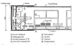
Figure 4 schematic section of a slurry shield Tunnel Boring Machine.
