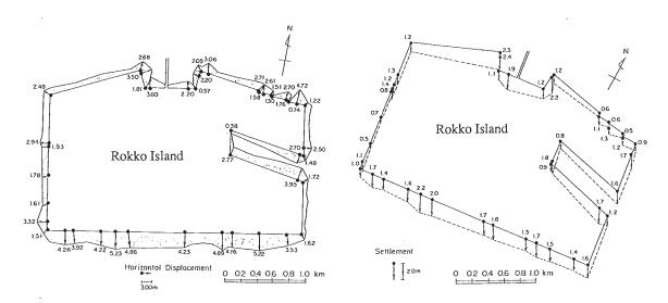
Figure 1 Horizontal and vertical movement of quaywalls on Rokko Island (after Inagaki et al 1996)...
