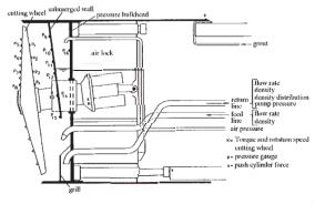
*Figure 6 Schematic overview of the total instrumention in the TBM.*
