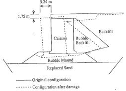
Figure 3 Typical effects of failure on quay walls.
