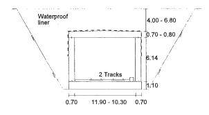
*Figure 2 Trench cut and cover method (all measures in metre).*
