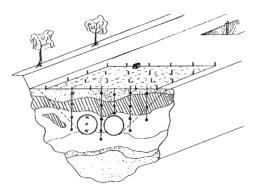
Figure 3 concept lay-out of the test area, in-situ earth and porewater pressure and subsidence marks on the surface.
