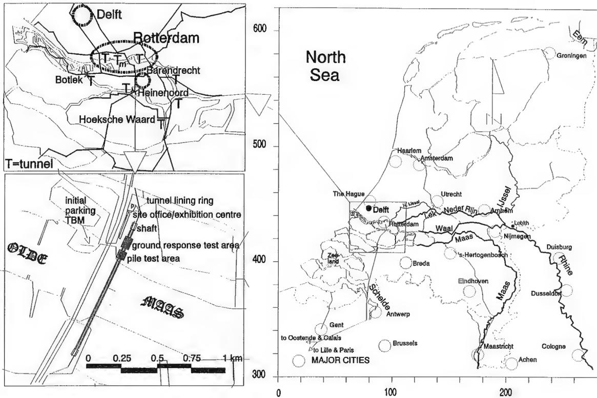
Figure 1 Location and plan of the Heinenoord tunnels including tunnel location around Rotterdam.
