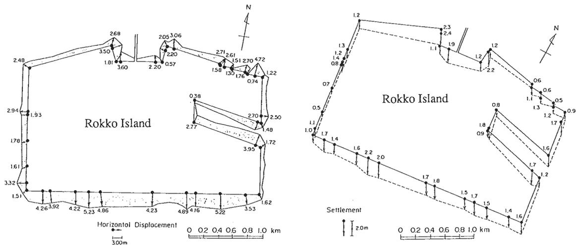
Figure 1 Horizontal and vertical movement of quaywalls on Rokko Island (after Inagaki et al 1996)..
