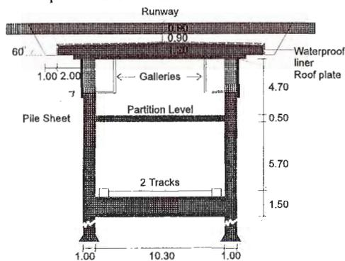
**Figure 3** Undercutting beneath a Sub-terrain Roof Plate (all measures in metre).
