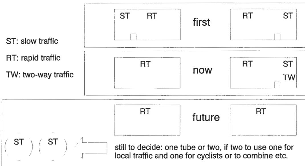
**Figure 7** Traffic configuration through first and second Heinenoord tunnels at various stages of use and development
