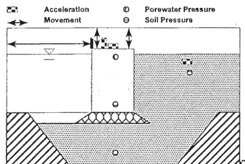
Figure 4 Arrangement of monitoring devices within centrifuge model.
