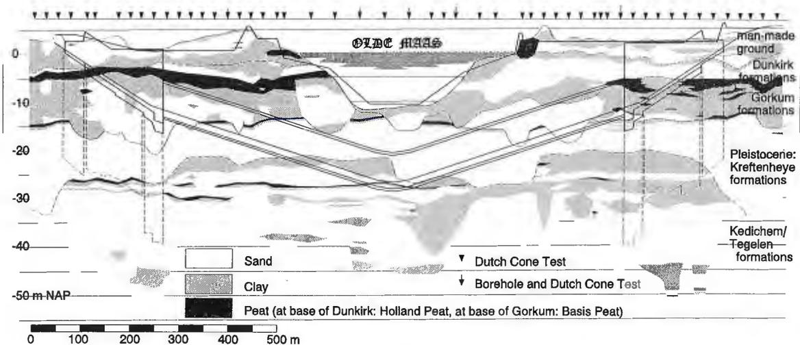
Figure 2 Geological profile and outline of second Heinenoord tunnel (note: anchor pile depths outlined beneath tunnel shaft and ramps).
