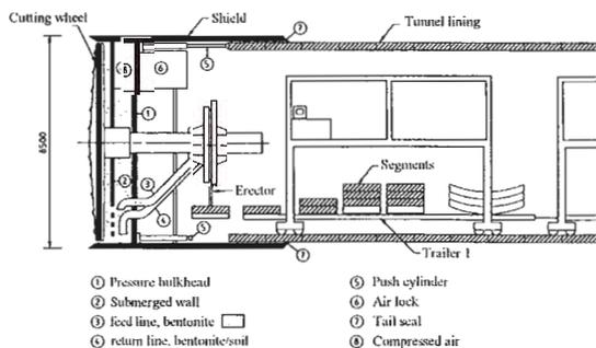
Figure 4 schematic section of a slurry shield Tunnel Boring Machine.
