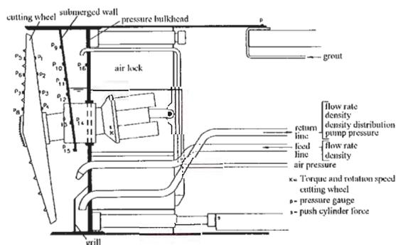
Figure 6 Schematic overview of the total instrumentation in the TBM.
