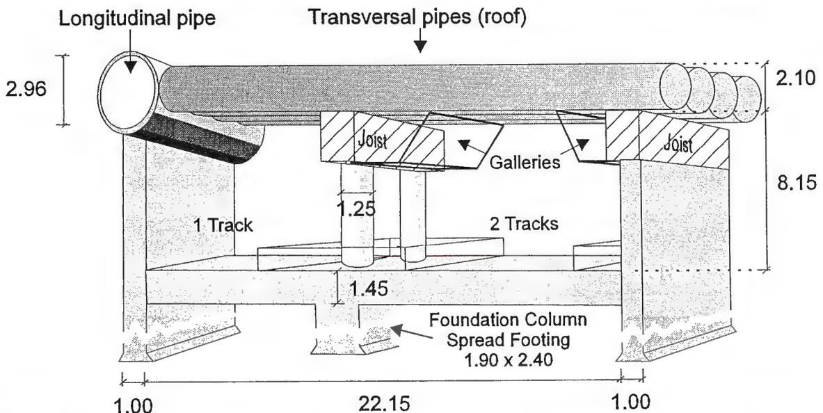
**Figure 6 Schematic view of the longitudinal and transversal pipes in the tunnel section C** (all measures in metre).
