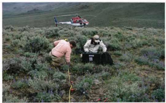
Seismic refraction survey used to forecast rock excavation for design of a pipeline in Humboldt County, NV.
