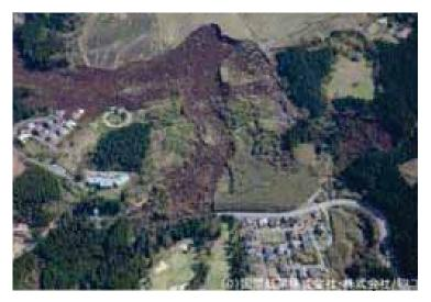
Fig.9 Landslide flows on gentle slope of the lava dome. Landslide slip would have occurred in the tephra which covered on the lava. (View from point B in the Fig.7)
