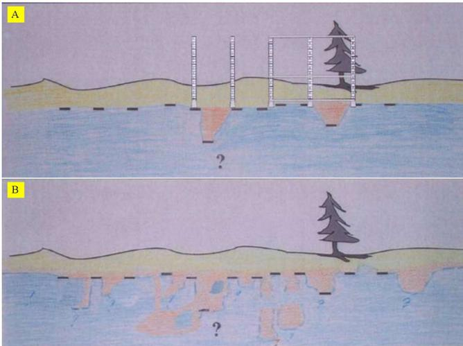
Figure 11. Conceptual model A and B. A is the engineering geological model of limited reality assumed to be correct in the 1980s. B represents the more realistic engineering geological model.
