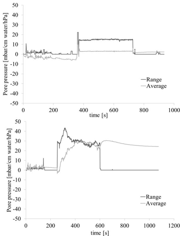
Figure 8. Pore pressure measurements during the penetrometer test on the Brazilian ore, below the FMP (top) and above the FMP (bottom).
