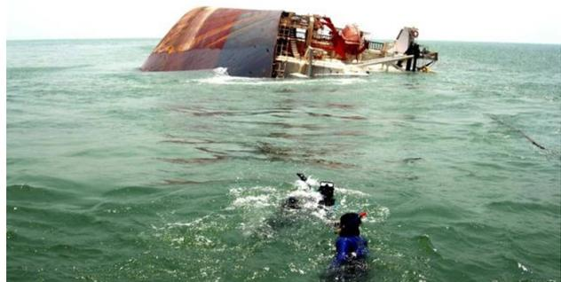
Figure 4 The MV Black Rose capsized as a result of cargo liquefaction on 9 September 2009. This incident triggered an international debate about the safety guidelines for the transportation of fine grained iron ores (The Hindu, 2009).
