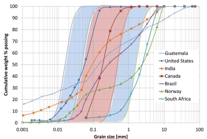
Figure 5. Grain size distributions of the ores provided by Oldendorff. Background colours indicate the ranges of grain size distributions which are highly susceptible to liquefaction (red) and potentially susceptible to liquefaction (blue) after Tushida (Terzaghi, 1996).
