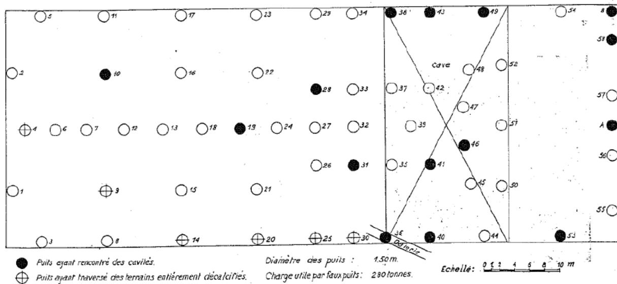
Figure 7. Location of 59 piles in the adapted foundation design. Black holes indicate where voids were encountered. Holes with crosses show where decalcified sandstone was encountered during the preparatory work for the 59 piles.
