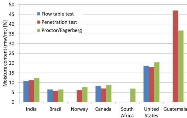
Figure 11 Results of the three TML tests
