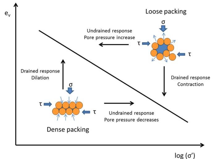
Figure 2. Susceptibility to liquefaction is related to the relative density of a material: Loosely packed granular materials tend to contract when loaded. Undrained conditions lead to an increase in pore pressure.
