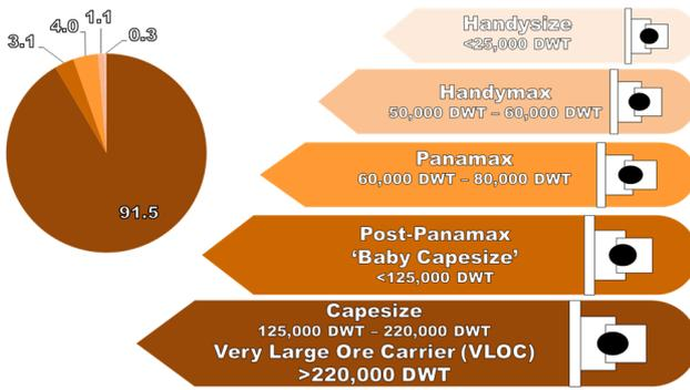
Figure 12 Different ship sizes and the amount of total iron ore transport divided over vessel type (after Stopford, 2002; IOTWG, 2013b)
