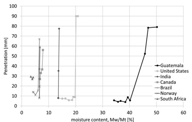
Figure 7. Results of the penetrometer test.
