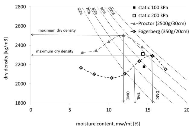
Figure 9; Compaction curves for Indian ores using different compaction methods: the tamping procedure of the FTT and PT applying a 'static' tamping pressure of 100 and 200 kPa; the original Proctor method using a hammer weight of 2500 g and drop height of 30 cm; and the modified method suggested by Fagerberg using a hammer weight of 350 g and drop height of 20 cm as prescribed in the IMSBC code (2009), the dashed lines indicate different degrees of saturation.
