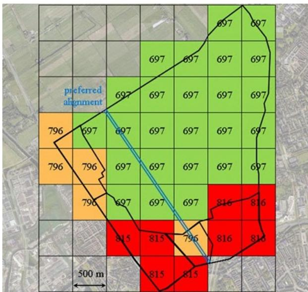
Figure 4. Whole life costs per 500x500 m<sup>2</sup> grid cell and preferred alignment of road.
