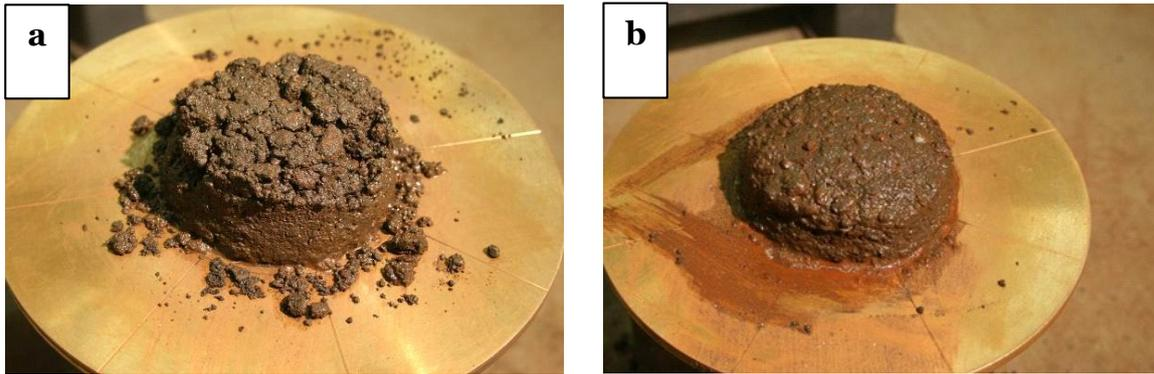
Figure 6. An example of the flow table tests performed on the Brazilian ore a) just below and b) just above FMP.
