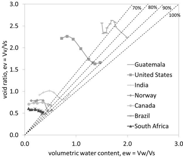
Figure 10. Results of the Proctor/Fagerberg tests. The dashed lines indicate different degrees of saturation.
