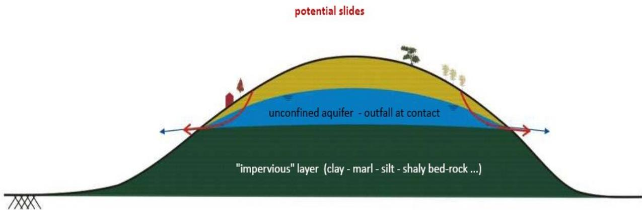
Figure 4. Conceptual engineering-geological model of the terrain on the basis of the geological map.
