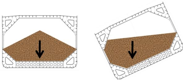
Figure 3. Shifting cargo displaces the vertical center of gravity of a ship and can cause the ship to capsize.
