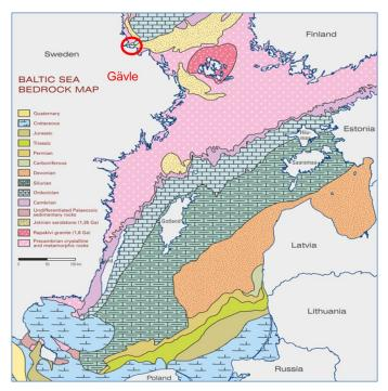
Figure 2: Geological bedrock map of the Baltic Sea (Tuuling et.al. 2011). Gavle harbour is positioned parallel to the late Precambrian fault system, Ordovician age limestone bedrock underlying glacial moraine with high boulder content had to be dredged in the access channel deepening project which was executed in 2012-2014.
