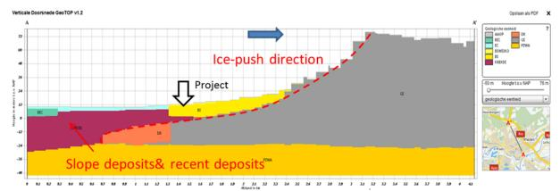
Figure 5 Project was located in the toe of an ice pushed ridge.
