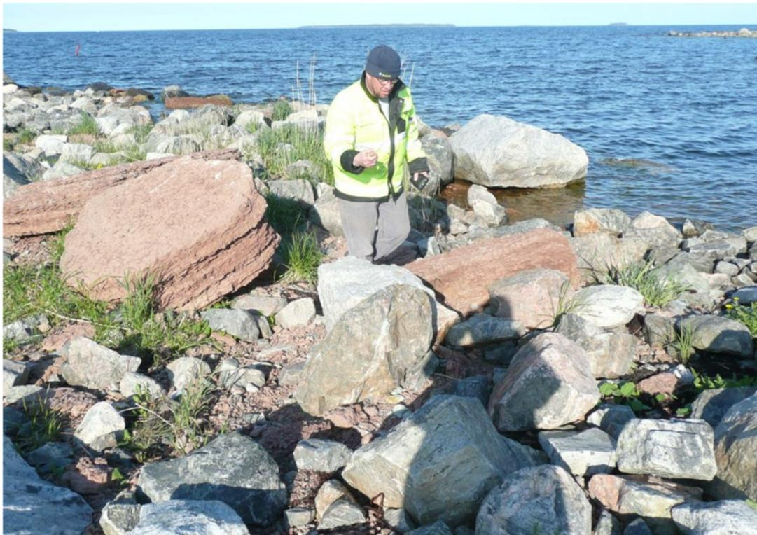
Figure 4: Gävle project. During the additional offshore ground investigations walk-over surveys were done along the coast using the geological maps. Locations were found where the red coloured limestone could be sampled for testing. Note the moraine boulders of hard crystalline rock which cover the limestone bedrock.
