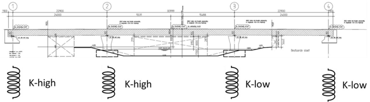
Figure 6 Variability in the stiffness below the bridge foundations.
