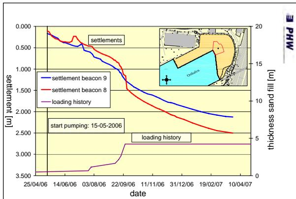
Figure 7 Typical time-settlement records observed after start of the pumps.
