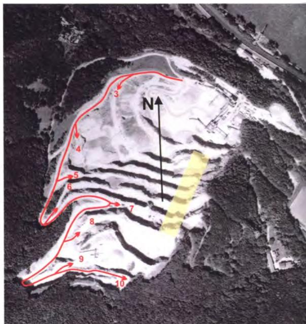
Figure 3 Ortho-photo of the Sooneck quarry in 2001, showing the preferred position of the pass in yellow. This preference is dictated by the road entrances to the bench levels.
