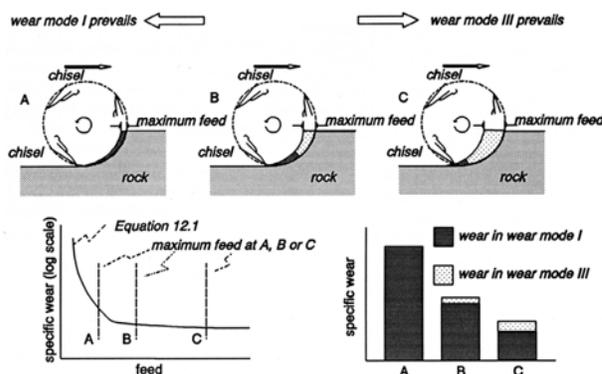
Figure 11 Cutter wear model of Deketh (Verhoef, 1997).
