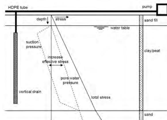
Figure 4 Principle of BeauDrain-S system including diagram of total, effective and pore water stresses.
