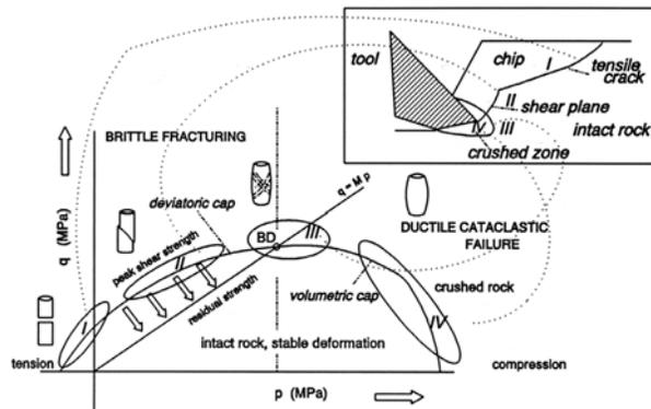
Figure 7 Model for the cutting of drag cutting tools into rock (Verhoef, 1997).
