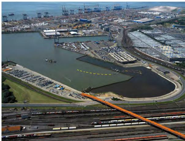
Figure 2 Overview of project during dredging operations (dredging pontoon, floating pipeline, and spreader pontoon).
