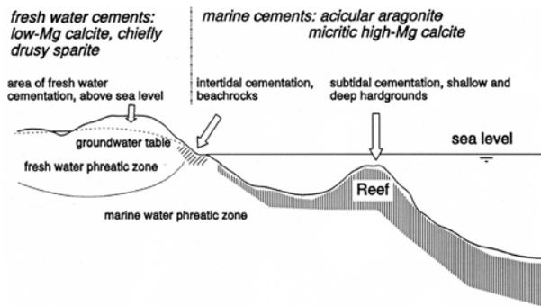
Figure 13 Cementation in coastal areas in the Middle East (Verhoef, 1997).
