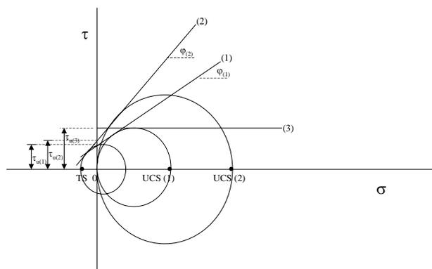
Figure 6 Failure envelope derived from the results of UCS and BTS tests. The ratio *m* (UCS/BTS) of rock (1)=5, of rock (2)=10. The failure envelope (3) is for porous rock tested under undrained conditions.
