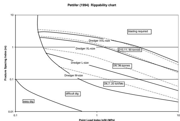
Figure 5 Pettifer diagram with conceptual boundaries for backhoe and hopper dredgers excavating rock. Boundaries have been chosen arbitrarily.
