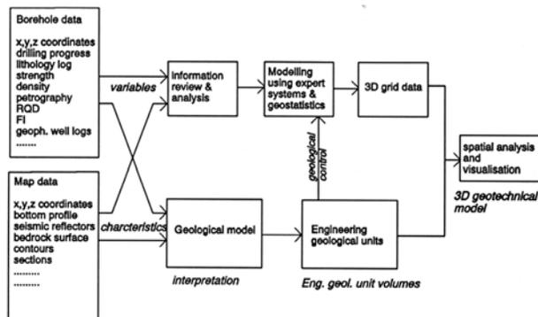
Figure 2 Flow diagram for the processing of data to arrive at a geotechnical model for the dredging of rock (Verhoef, 1997).
