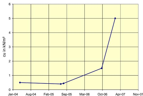
Figure 6 Increase of average undrained shear strength with time.
