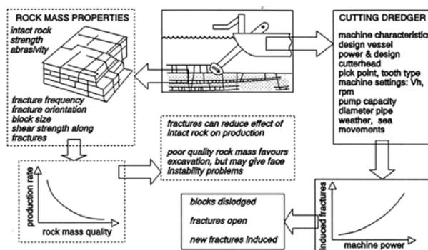
Figure 3 Interaction between rock mass and excavation tool (Verhoef, 1997).
