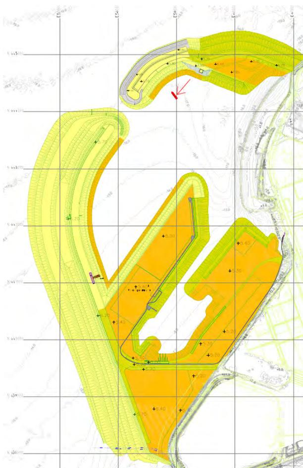
Figure 1 Top view of the MV 2 project under construction. The coloured areas are being reclaimed with different types of sand. Red arrow indicates location of TSHD Oranje as visited by the author on 30 July 2010 (see Figure 2).
