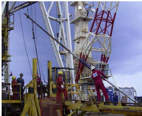
Figure 4 Pressure corer handling. The pressure corer (FRPC) is hoisted into the derrick to be lowered in the drill string. The drill string acts as casing during the pressure coring operations (courtesy of Fugro).
