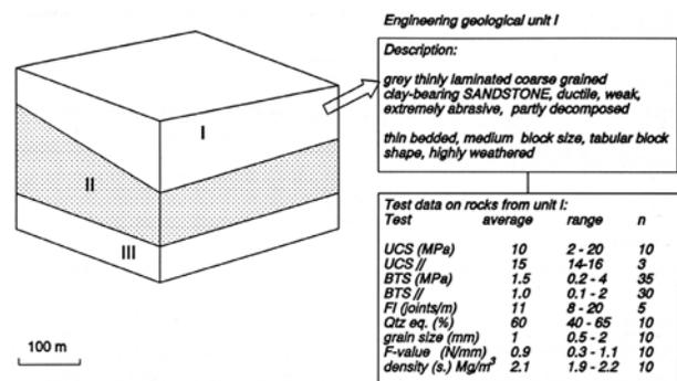
Figure 1 Geotechnical model with engineering geological units (Verhoef, 1997).
