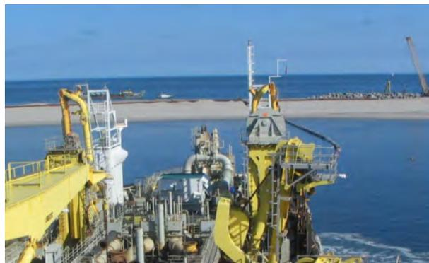
Figure 2 TSHD Oranje, pumping sand (deposited between 100,000-300,000 yrs ago) ashore via a floating line, thereby reclaiming the outer MV 2 area from sea.
