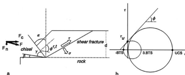
Figure 9 a) Model for shear failure by Nishimatsu; b) Method to calculate  $\tau_u$  using UCS and BTS (Verhoef, 1997).
