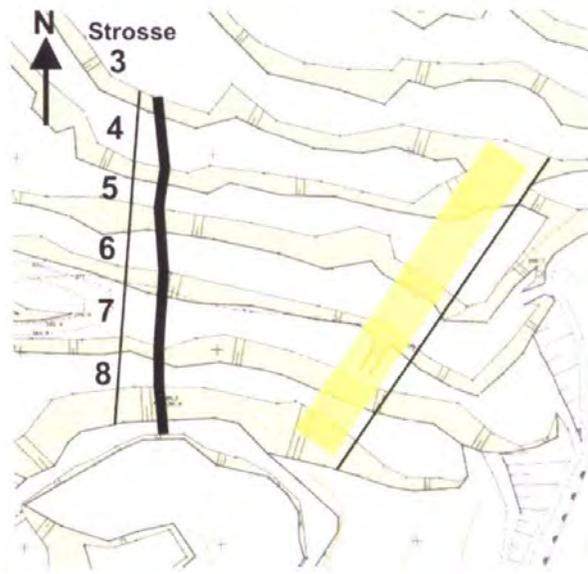
Figure 4 The black line on the left shows the best position for an ore pass based on the SSPC analysis by Xander van Beusekom in 1999.
