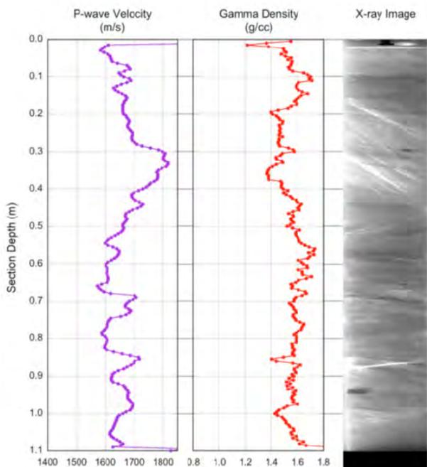
Figure 3 Non-destructive measurements on a pressure core. X-ray image shows gas hydrate (white) morphology in clay (grey). Note the complex structure of fine veins. Where gas hydrate is present, the P-wave velocity is higher and the gamma density is lower than where gas hydrate is absent (courtesy of GeoTek).
