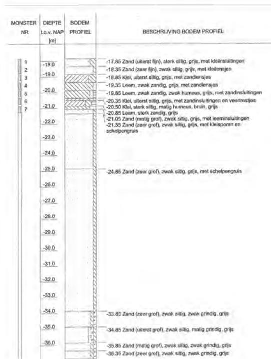
Figure 5 Borehole log representing the different sediments and depths. First used for engineering purposes, later on to determine the historic time period.
