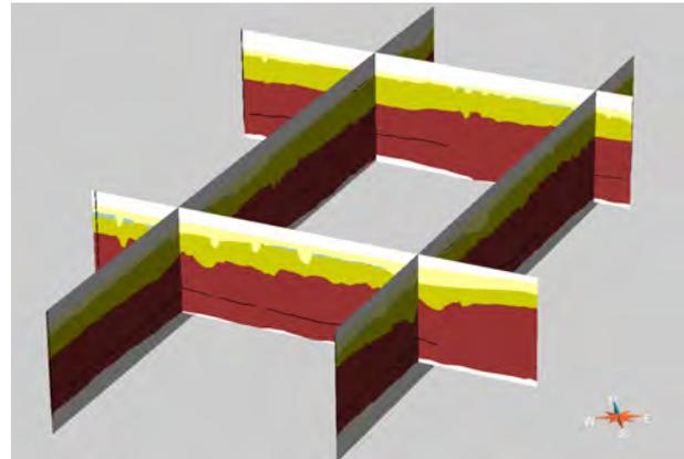
Figure 4 Visualisation of the 3D soil model of MV2 (brown layer represents the Kreftenheye Formation).
