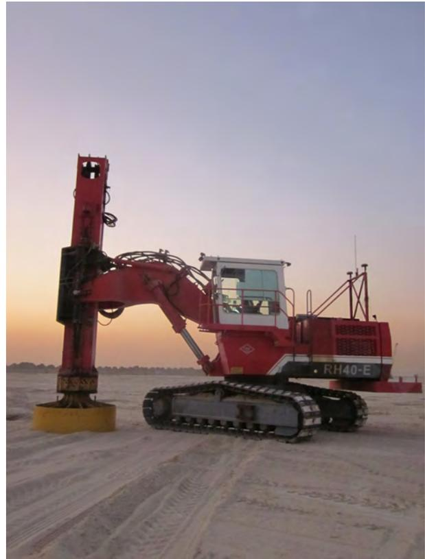
Figure 2 CDC machine (O&K RH40) in action.
