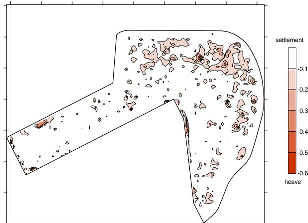
Figure 3 Result of a bathymetric survey of the fill surface after occurrence of deformations.
