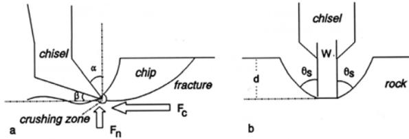
Figure 8 a) Evans' model for the cutting of rock with drag cutting tools; b) This figure shows the outbreak geometry of chips with characteristic outbreak angle  $\theta_s$  (Verhoef, 1997).
