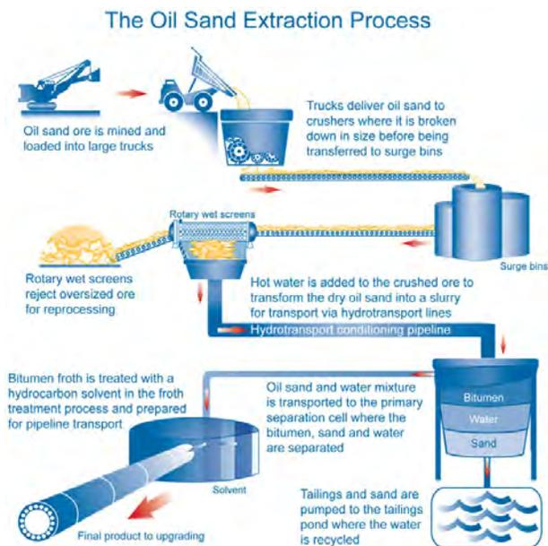
Figure 4 Schematisation of the oil sands extraction process (Hatch, 2008).
