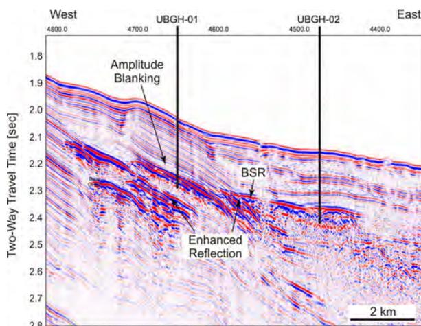
Figure 2 Gas hydrate indicators on seismic data. Bottom-simulating reflector (BSR) is associated with the interface between gas hydrate (above) and gas (below). The depth of the BSR corresponds to the depth of the base GHSZ, which is defined by the geothermal gradient. Gas appears as enhanced reflections and gas hydrate as blanked amplitude reflections in this section. Example is taken from the Ulleung Basin in the East Sea between South Korea and Japan (courtesy of KNOC).
