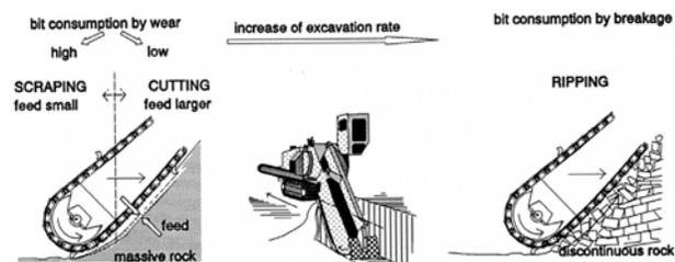
Figure 10 Transition from cutting to ripping for a rock cutting trencher (Verhoef, 1997).
