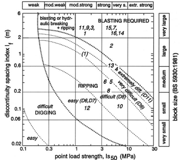
Figure 4 Rippability chart of Pettifer & Fookes (1994). This chart is based on 120 cases of ripping with Caterpillar bulldozers. The numbers in the plot refer to projects with Vermeer T850 trenchers, which are reported in Verhoef (1997).
