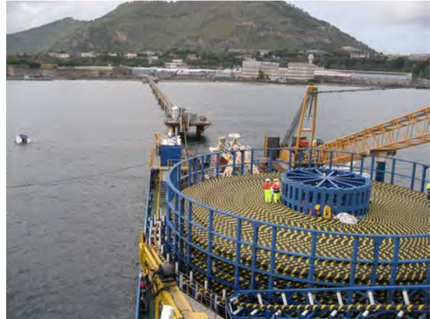
Figure 2 Loading a power cable.
