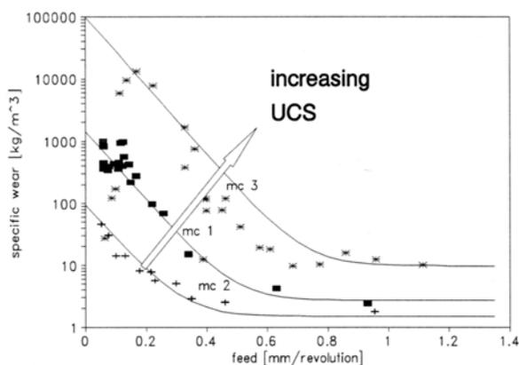
Figure 12 Specific wear against cutting depth (feed) of chisels cutting in artificial quartz concrete with a UCS of 18 MPa (mc 2), 30 MPa (mc 1) and 68 MPa (mc 3); cutting velocity of all tests 0.4 m/s (Deketh 1995).
