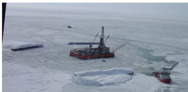
Figure 10 Exploration drilling barge protected by four IPS.
