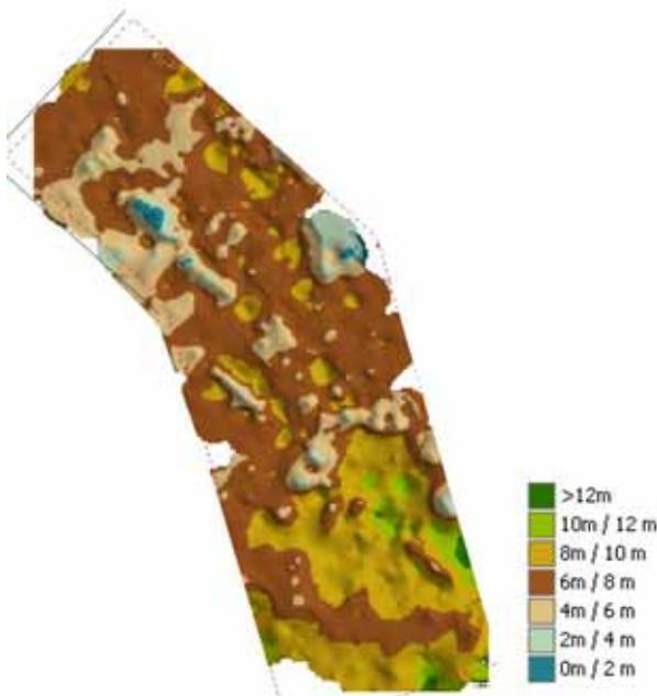
Fig. 5 Thickness of dredgeable sediments ( $V_p < 2,150$  m/s) from a GAMBAS<sup>®</sup>50 survey at Banyan terminal (Singapore) (Map computed with ArcGIS<sup>®</sup> 9).
