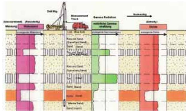
Fig. 4 Typical lithology encountered in the Rhenish lignite mining district and the readout on a schematic geophysical log.
