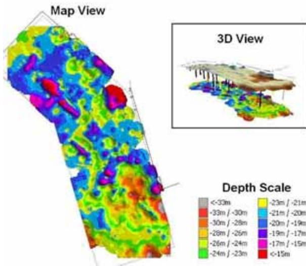
Fig. 6 Depth of substratum, i.e.: seismic velocities above 2,150 m/s from a GAMBAS<sup>®</sup>50 survey at Banyan terminal (Singapore) (Map and 3D view (sea bed, substratum and boreholes) computed with ArcGIS<sup>®</sup> 9).
