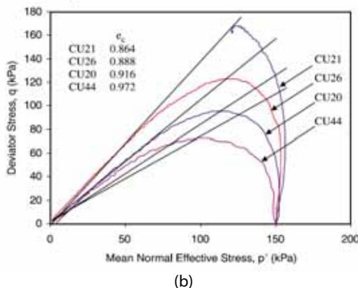
Fig. 2 a) Location of instability line for loose sand (Fig. 7 from Lade (1992)); b) Variation of instability line with varying void ratio after consolidation  $e_c$  (Fig. 3 from Chu et al. (2003)).
