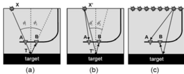
Fig. 2 Example to illustrate the concepts of seismic interferometry: a) source located at X; b) source located at X' (right of X); c) multiple source locations.
