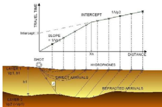
Fig. 1 Basic refraction principle.
