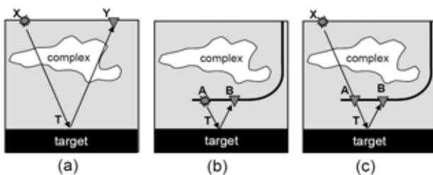
Fig. 1 Imaging below complex overburden: a) conventional acquisition design with sources and receivers at the earth's surface, located at X and Y, respectively; b) desired acquisition, with sources and receivers in a borehole, located at A and B, respectively; c) acquisition for seismic interferometry, with sources at earth's surface location X and receivers in the borehole at locations A and B, where location A corresponds to the virtual source location.
