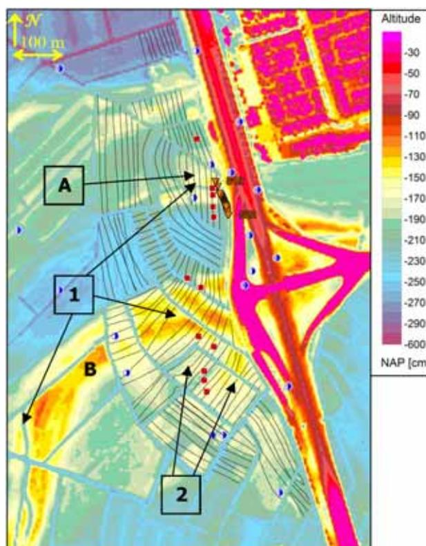
Fig. 5 Airborne surface elevation map with GEM-2 survey tracks in black. Orange triangles: Delft Cluster CPT's. Blue dots: archived boreholes. Red squares: hand-made gauge boreholes. The capital letters and numbers are explained in the text.
