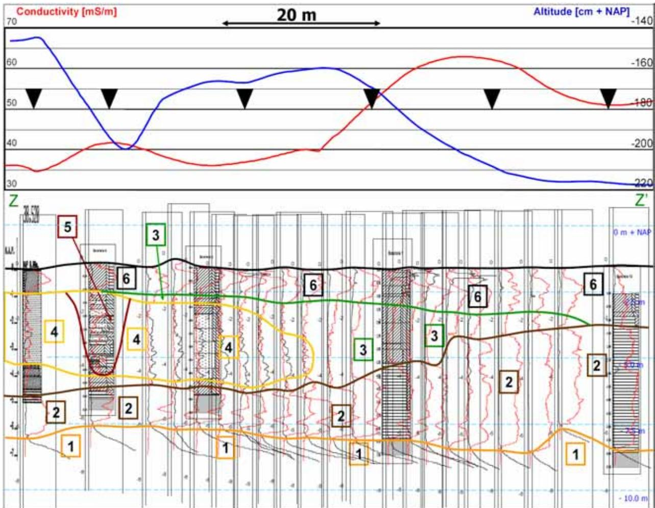
Fig. 7 Geotechnical profile Z-Z' compared to GEM-2 total conductivity profile (red line in mS/m) and a surface elevation profile (blue line in cm relative to NAP).
