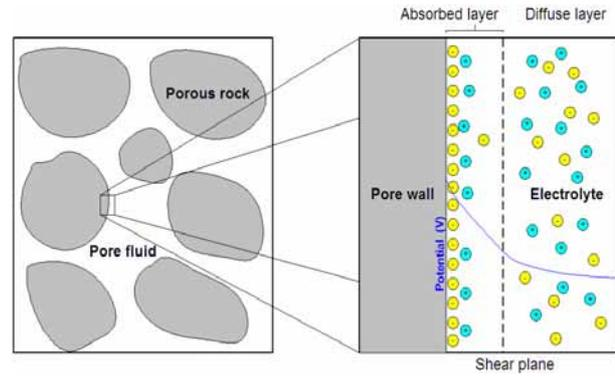
Fig. 1 The electric double layer.
