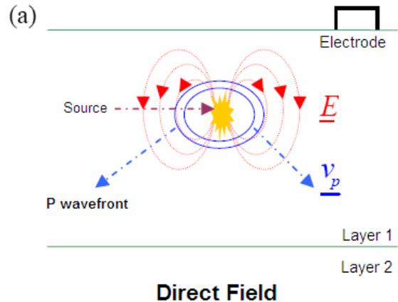
Fig. 4a Seismo-electric effects: direct field (Haines, 2004).
