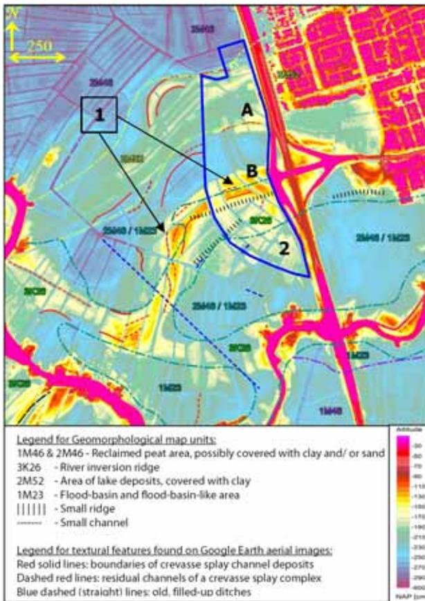
Fig. 4 Geomorphological unit boundaries (dash-dotted lines) superimposed on an airborne laser altimetry map, and combined with textural features found on Google Earth images. Unit codes and textural features are explained in the legend. Blue line: pilot site. A and B: main crevasse channels. The numbers are explained in the text. Note: elevation is in centimetres relative to NAP, and a larger scale is shown in Figure 5.
