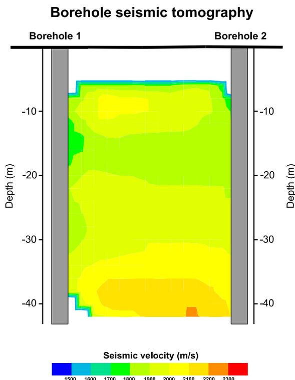
Fig. 7 Preliminary results from crosshole seismics between boreholes 1 and 2.
