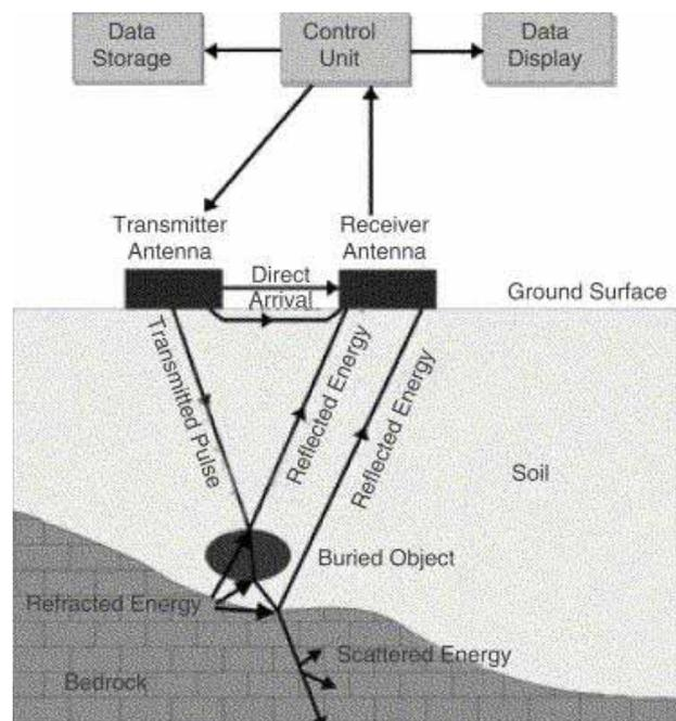
Fig.1 Schematic representation of GPR data-acquisition.
