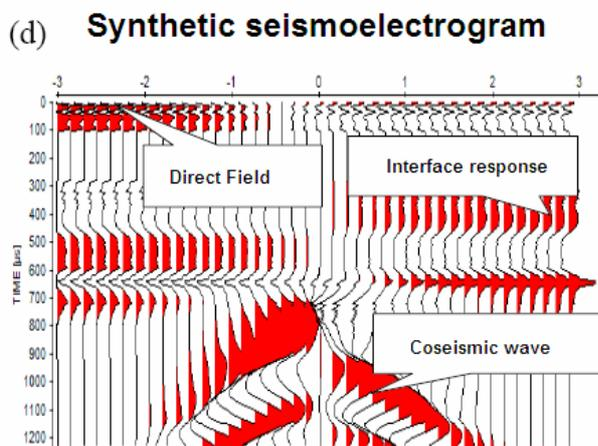
Fig. 4d Seismo-electric effects: seismo-electrogram (Haines, 2004).
