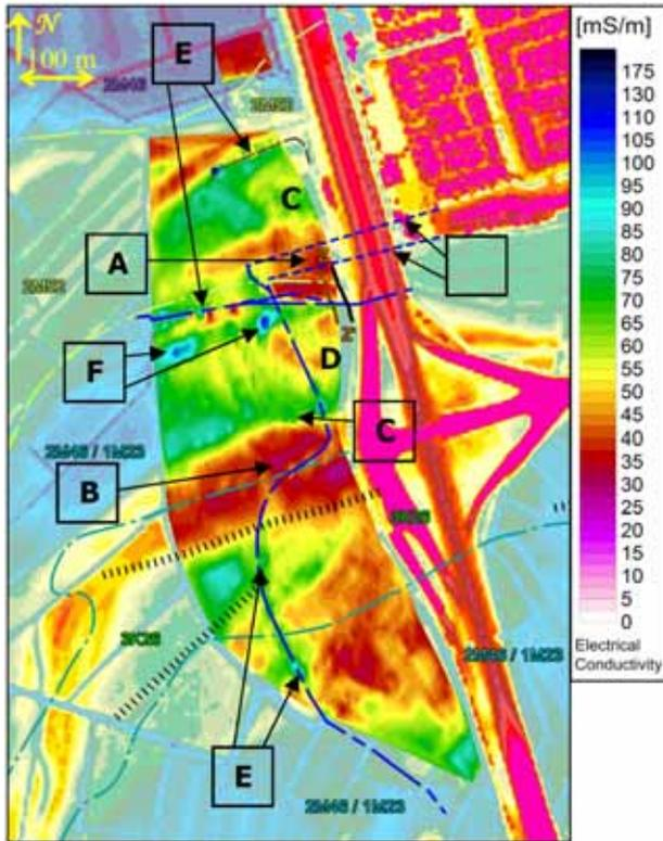
Fig. 6 GEM-2 total conductivity map superimposed onto the surface elevation map with geomorphological unit boundaries (long dash-dotted line). Blue long dash-short dashed line: telephone cables. Blue short dashed line: horizontally drilled cables under motorway. Grey dashed line: reinforced concrete path. Black solid line: geotechnical profile Z - Z'. Brown solid line: surface elevations and GEM-2 profiles for Figure 7. Capital letters are explained in the text.
