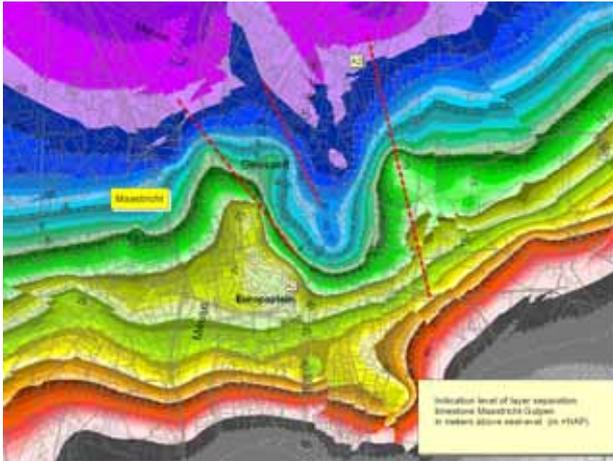
Fig. 2 Fault lines and top of Gulpen Formation, based on boreholes.
