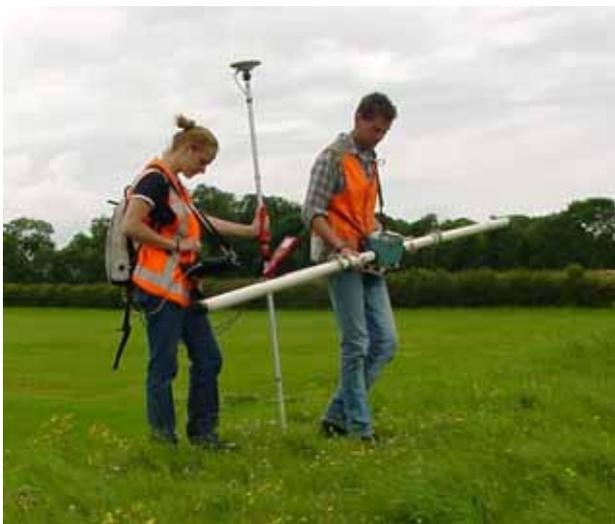
Fig. 4 EM-meter and GPS-receiver.
