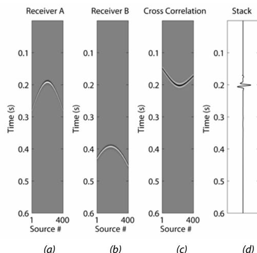
Fig. 4 400 shot positions: a) direct wave at A; b) scattered wave at B; c) cross-correlation functions; d) stack of cross-correlation functions.
