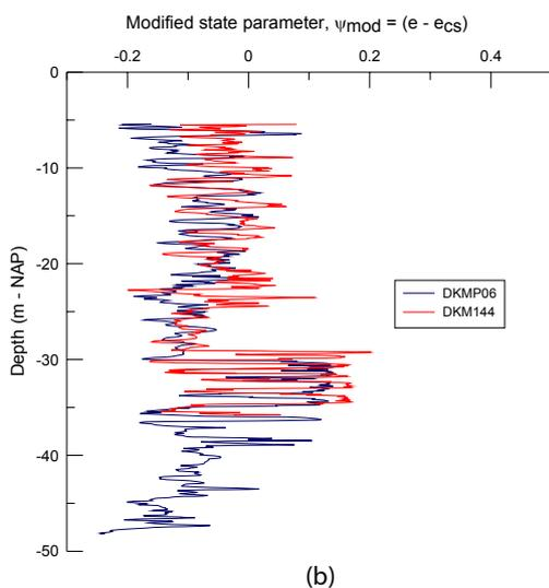
Fig.4 a) Underwater survey of dike failure of August 26th, 2007 (~350.000 m<sup>3</sup>) (source: Combination Sassenplaat); b) Modified state parameter profile at failure location.
