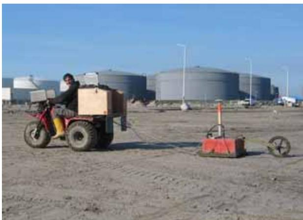
Fig. 5 200 MHz GPR antenna (orange box), with GPS receiver mounted on top, measuring at the Europoort site.
