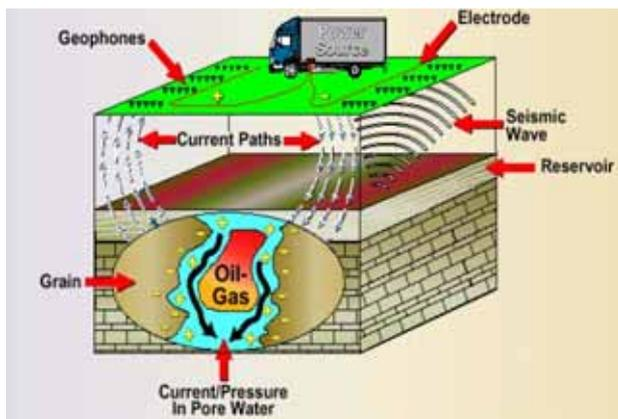
Fig. 5 Electro seismic prospecting in the field.
