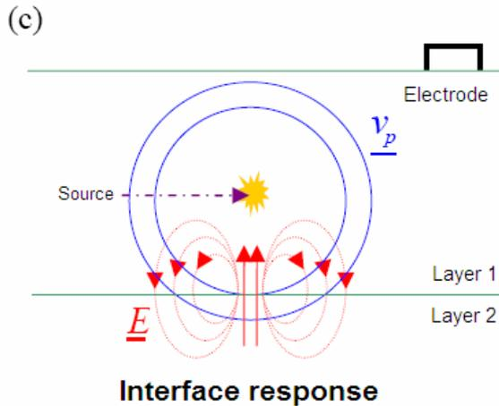
Fig. 4c Seismo-electric effects: interface response (Haines, 2004).
