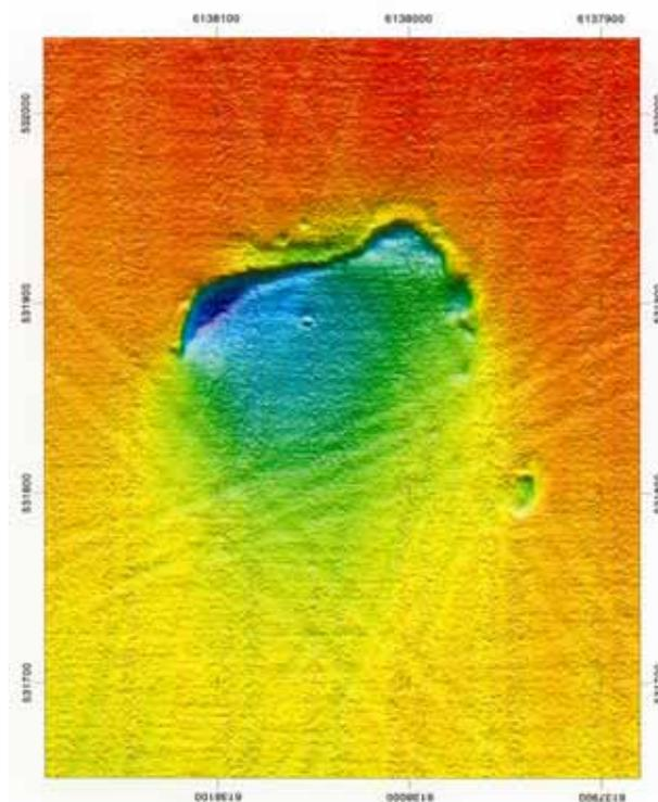
Fig. 2 Multibeam image of a pock mark in block A11 in the Dutch sector, with a diameter of about 150 m. The wall of sediment left behind after the explosion is still partly visible. Trawling scars have destroyed the pockmark partly.
