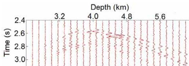
Fig. 6 Redatumed virtual shot record with seismic interferometry by multi-dimensional deconvolution (red) superimposed on a reference response, generated by placing an active source at the virtual source location (black).
