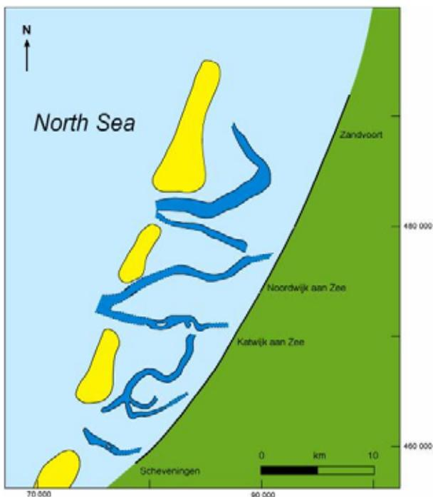
Fig. 5 The pattern of offshore Holocene tidal channels mapped with high resolution seismics west of the coast of South Holland.
