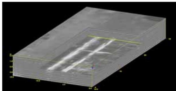
Fig. 6 3D image of the processed GPR data showing several pipes at a certain depth.
