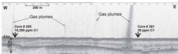
Fig. 4 Gas seeps in block B13 of the Dutch sector. Cores taken near the plumes revealed anomalies of 39 vppm CH<sub>4</sub> at a depth of 3.5 m below sea bed.
