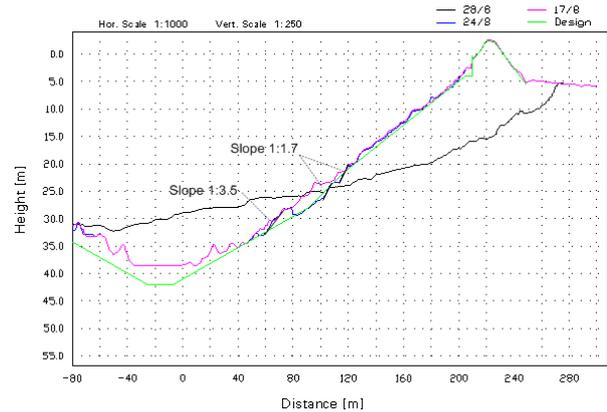
Fig.5 Graphical representation of cross-section dike failure August 26th, 2007 and design slope, constructed slope and slope after instability (source: Combination Sassenplaat).
