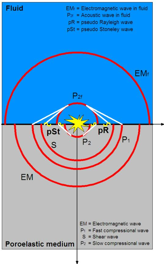
Fig. 3 Characteristic waves in half space at fluid/poro-elastic medium boundary. The 4 characteristic waves and some surface waves (Rayleigh and Stoneley) are shown.
