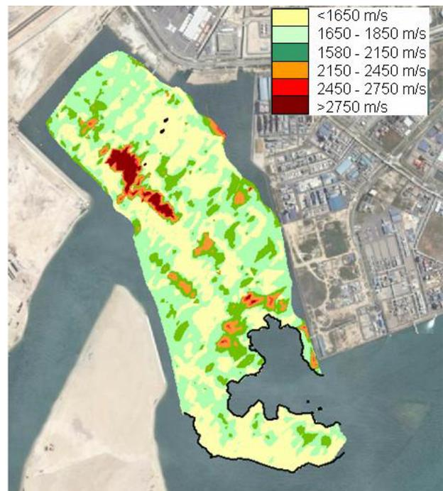
Fig. 4 Distribution of velocity classes at -18 m LAT (target depth) from a GAMBAS®50 survey at Banyan terminal (Singapore) (Map computed with ArcGIS® 9).
