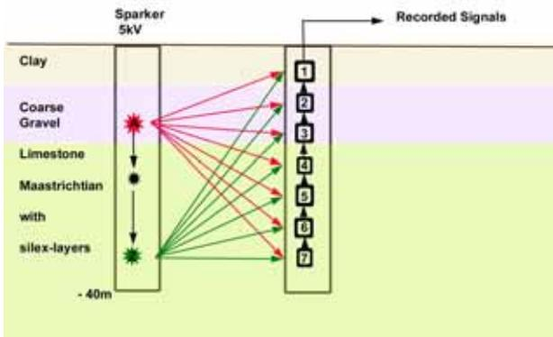
Fig. 6 Principle of crosshole seismics.
