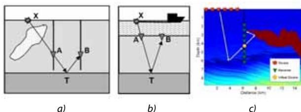
Fig. 5 a) generating virtual crosswell data; b) ocean bottom cable redatuming; c) salt flank imaging.
