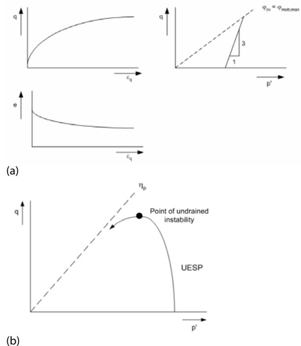
Fig. 1 a) Drained behaviour of strongly contractive soils (triaxial loading); b) Undrained effective stress path (UESP) and resulting liquefaction.
