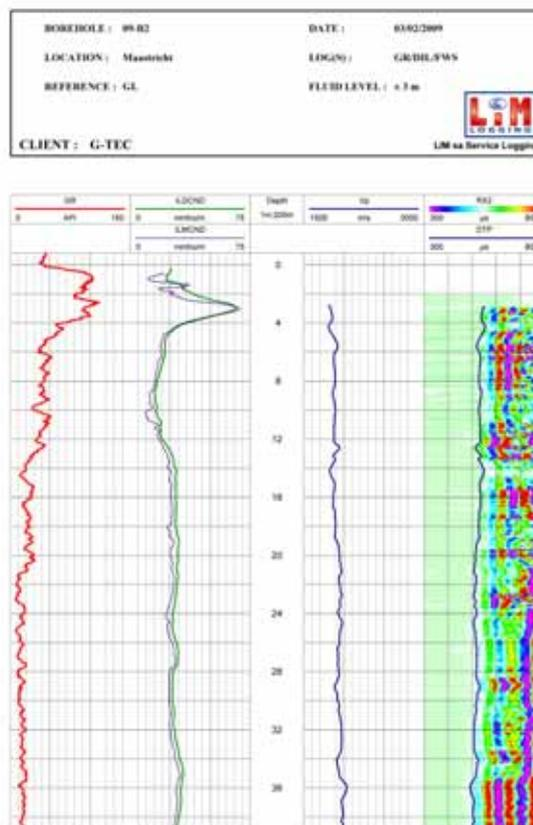
Fig. 5 Results from logging of borehole 2 (without geological interpretation).
