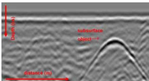
Fig. 2 Radargram showing the hyperbola-shaped reflection caused by a subsurface object.
