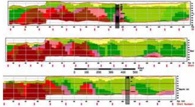
Fig. 3 Example of a velocity profile, correlated with geotechnical bore-holes (computed with StarfixGambas®).
