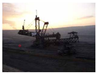
Fig. 2. The standard bucket wheel excavator in Hambach surface mine. The encircled Land Rover serves as scale.
