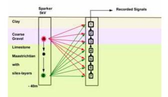
Fig. 6 Principle of crosshole seismics.
