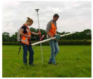
Fig. 4 EM-meter and GPS-receiver.
