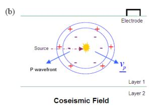
Fig. 4b Seismo-electric effects: coseismic field (Haines, 2004).
