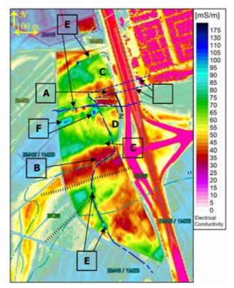
Fig. 6 GEM-2 total conductivity map superimposed onto the surface elevation map with geomorphological unit boundaries (long dash-dotted line). Blue long dash-short dashed line: telephone cables. Blue short dashed line: horizontally drilled cables under motorway. Grey dashed line: reinforced concrete path. Black solid line: geotechnical profile Z - Z'. Brown solid line: surface elevations and GEM-2 profiles for Figure 7. Capital letters are explained in the text.
