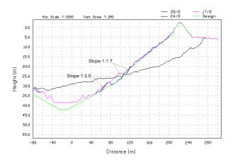
Fig. 5 Graphical representation of cross-section dike failure August 26th, 2007 and design slope, constructed slope and slope after instability (source: Combination Sassenplaat).
