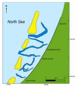
Fig. 5 The pattern of offshore Holocene tidal channels mapped with high resolution seismics west of the coast of South Holland.
