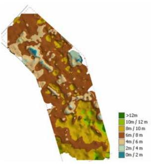
Fig. 5 Thickness of dredgeable sediments (V<sub>p</sub> < 2,150 m/s) from a GAM-BAS\*50 survey at Banyan terminal (Singapore) (Map computed with ArcGIS\* 9).
