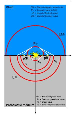
Fig. 3 Characteristic waves in half space at fluid/poro-elastic medium boundary. The 4 characteristic waves and some surface waves (Rayleigh and Stoneley) are shown.
