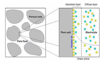
*Fig.* 1 *The electric double layer.*
