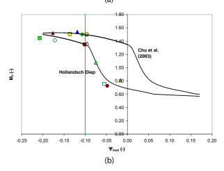
Fig. 3 a) Artist impression of dredge sludge depot Hollandsch Diep; b) Laboratory data of Modified State parameter versus slope of instability line  $M_{lL}$  (=q/p').
