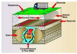
Fig. 5 Electroseismic prospecting in the field.
