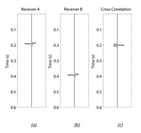
Fig. 3 Seismic traces: a) direct wave at A; b) scattered wave at B; c) cross-correlation function.
