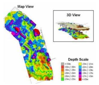
Fig. 6 Depth of substratum, i.e.: seismic velocities above 2,150 m/s from a GAMBAS\*50 survey at Banyan terminal (Singapore) (Map and 3D view (sea bed, substratum and boreholes) computed with ArcGIS\*9).
