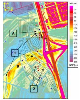
Fig. 5 Airborne surface elevation map with GEM-2 survey tracks in black. Orange triangles: Delft Cluster CPT's. Blue dots: archived boreholes. Red squares: hand-made gauge boreholes. The capital letters and numbers are explained in the text.
