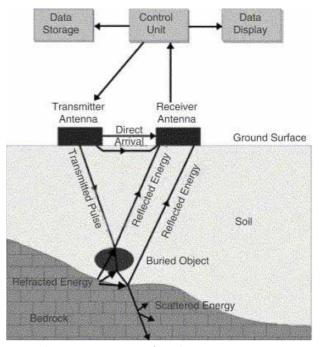
Fig.1 Schematic representation of GPR data-acquisition.
