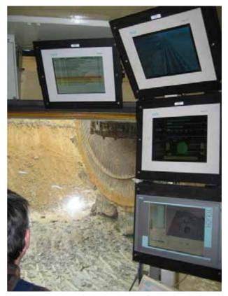
Fig. 2 The IT-system inside the control room of the bucket wheel excavator (photo by Arjan Kochx).
