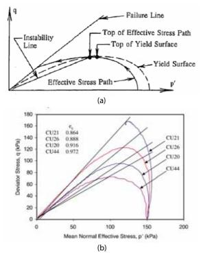
Fig. 2 a) Location of instability line for loose sand (Fig. 7 from Lade (1992)); b) Variation of instability line with varying void ratio after consolidation  $e_c$  (Fig. 3 from Chu et al. (2003)).
