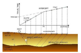
*Fig.* 1 *Basic refraction principle.*
