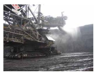
Fig. 1 The 90 m high bucket wheel excavator excavating grey, clayey soil (photo by Arjan Kochx).
