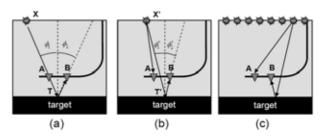
Fig. 2 Example to illustrate the concepts of seismic interferometry: a) source located at X; b) source located at X' (right of X); c) multiple source locations.
