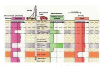
Fig. 4 Typical lithology encountered in the Rhenish lignite mining district and the readout on a schematic geophysical log.
