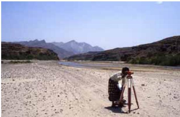
Fig. 6 Levelling at run-off measuring station, Wadi Adhanah.
