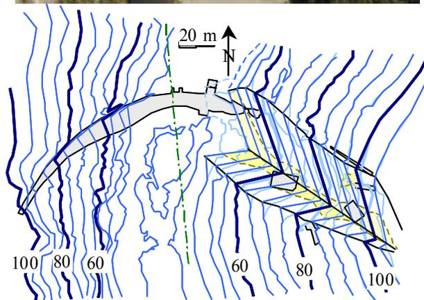
Fig. 2 Photograph and contour map of Malpasset Dam site after failure showing tie-in between wedge contours and ground contours; shaded portion is wedge. Wedge contours below survey contours (ground surface) indicating P3 either at a higher elevation or probably P3 consists of two or more planes (photo source: en.structurae.de/photos/index.cfm?JS=7596; photo used with permission of photographer Alain de la Forest (alaindelaforest@yahoo.fr)).
