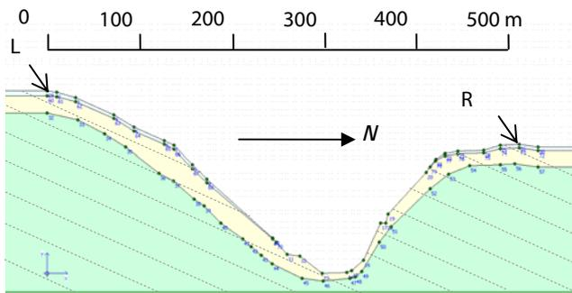
Fig. 3 Measurement points at the slope crests, L: left, R: right (equal horizontal and vertical scales) and apparent dip of the layers.
