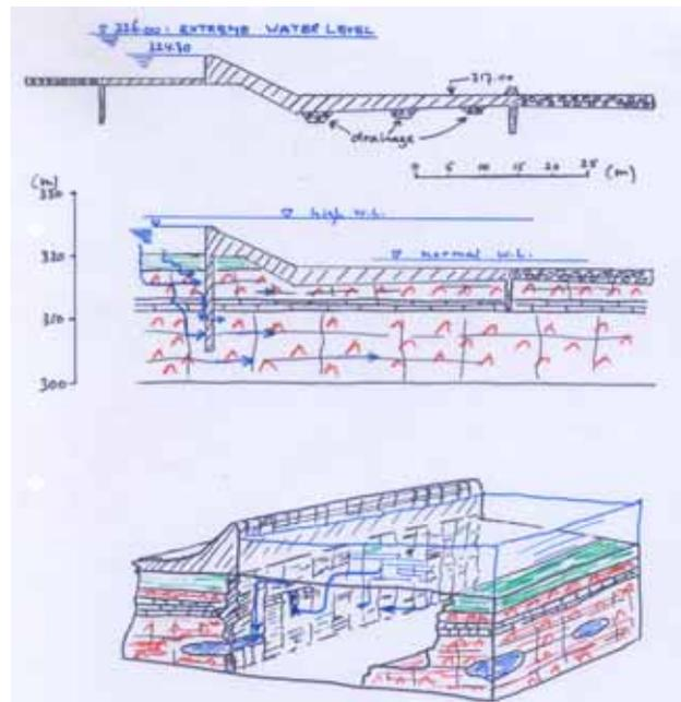
Fig. 12 Sketch of the design of the diversion weir and hypothetical drawings of the groundwater flow paths in the case of a design with a grout curtain. The disadvantage of a grout curtain is the possibility of dissolution taking place right at the dam structure itself.
