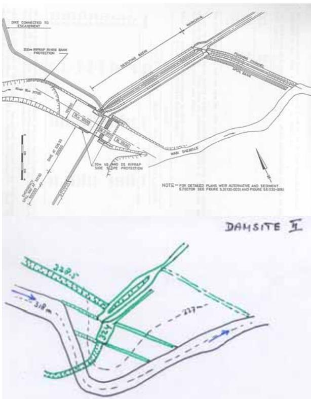
Fig. 10a: design of the diversion weir (top); 10b: sketch map (bottom).
