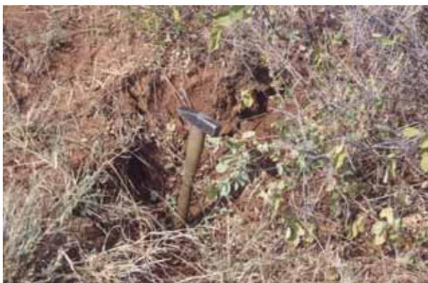
*Photo 6 Sinkhole about 40 cm deep, developed after rainy period of two weeks.*
