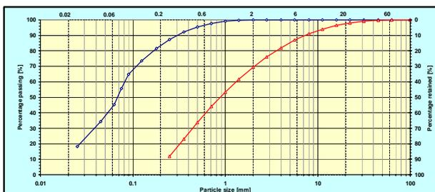
Fig. 5 Grain size distribution range of piped soils.
