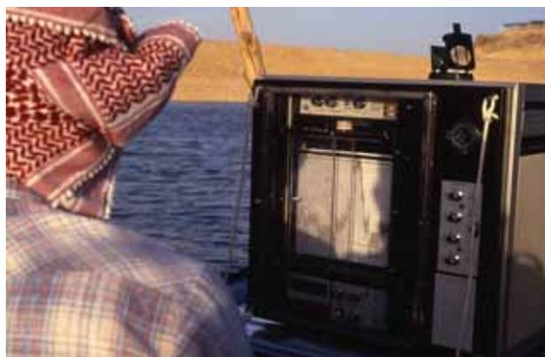
Fig. 3 Marib Dam and reservoir with survey boat (top), seismic reflection sediment sub-bottom profiler (bottom).
