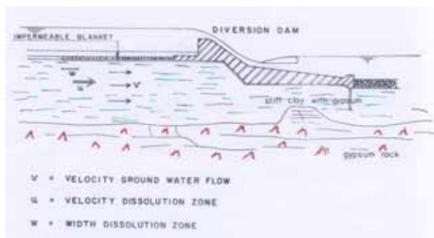
Fig. 13 Design of the diversion weir on stiff clay with impermeable blanket.
