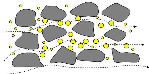
Fig. 1 Piping phenomenon: transport of fine soil (fine sand) amongst coarse particles (gravel).
