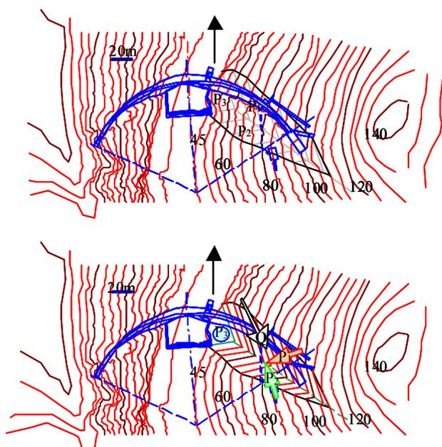
Fig. 1 Contour map prior to failure showing the plan of the dam and the underlying wedge causing failure. Contour map based on Londe (1987), wedge based on Londe, Vigier and Vormeringer (1970).
