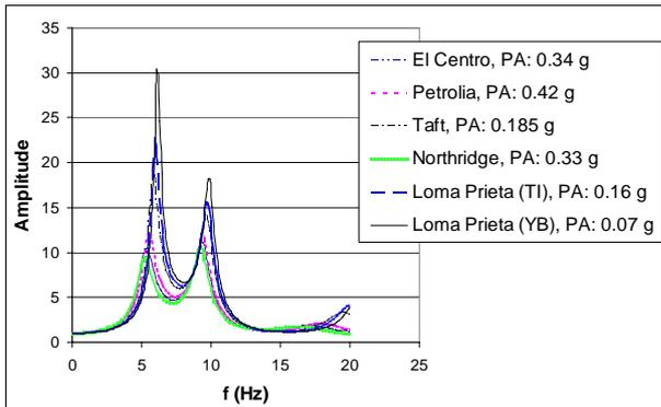
Fig. 4 Oscillation modes at the accelerograph location on the right slope.
