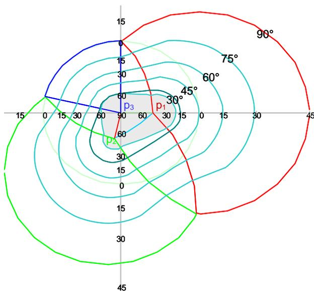
Fig. 5 Friction 'cones' added to show increased safe zone. Values correspond to Londe (1973) and are 25°, 15° and 30° for shaded zone. Friction angle iso-lines plotted for 30° through 90°.
