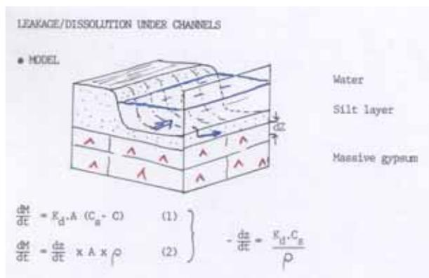
Fig. 14 Concept of dissolution of unlined irrigation canal above gypsum rock.
