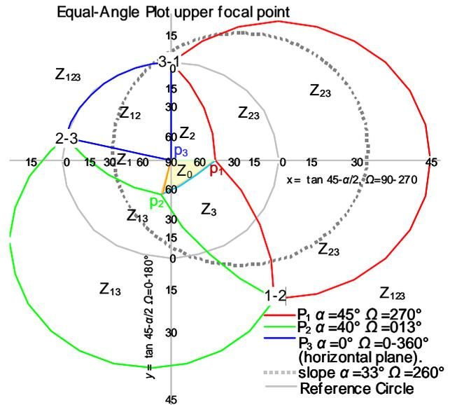
Fig. 4 Continuation of Figure 3, using a spreadsheet connecting poles of P1, P2 and P3 ( $p_1$ ,  $p_2$  &  $p_3$ ) with intersection points of P1-P2, P2-P3 and P3-P1 (1-2, 2-3 & 3-1) Londe rupture modes  $Z_0$  through  $Z_{123}$  shown. A force in a direction within zone  $Z_0$  is considered as safe.
