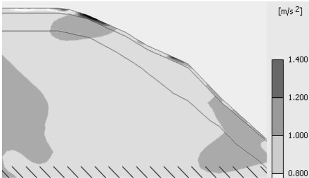
Fig. 6 Peak horizontal accelerations on the left slope (in  $m/s^2$ ). Peak towards the crest. Response under the motion of December 28, 2005.
