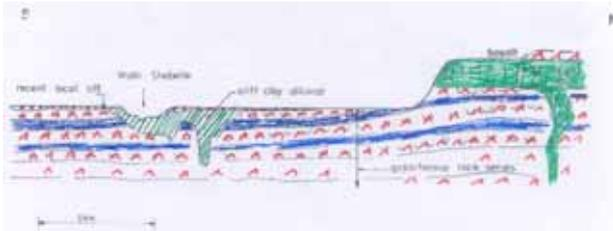
Fig. 11 NS geological cross section through the valley of the Wabi Shebelle.
