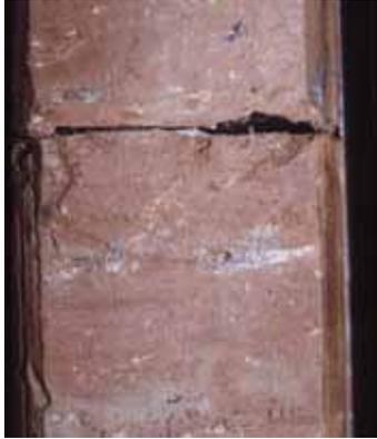
Photo 4 120 mm tube core of stiff clay with gypsum veins and nodules (borehole H).
