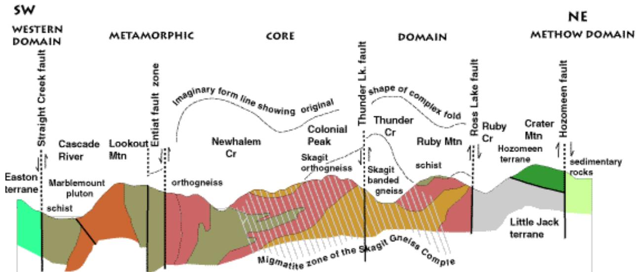
Fig. 12 Cross sectional sketch of giant fold exposing migmatites in the Metamorphic Core Domain (Chelan Mountains terrane) (source: [www2.nature.nps.gov/GEOLOGY/usgsnps/noca/nocastc.html#Napeeqa](http://www2.nature.nps.gov/GEOLOGY/usgsnps/noca/nocastc.html#Napeeqa)).
