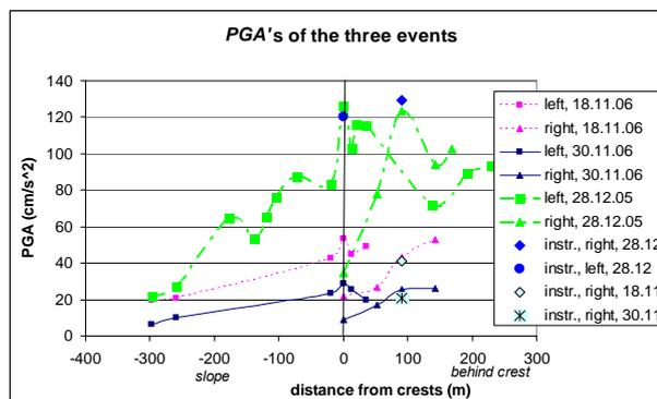
Fig. 5 Peak ground accelerations of the three motions along the left slope and behind the crests of both slopes. The zero on the x-axis represents the crest of each slope. "Instr." are the instrumental field measurements.
