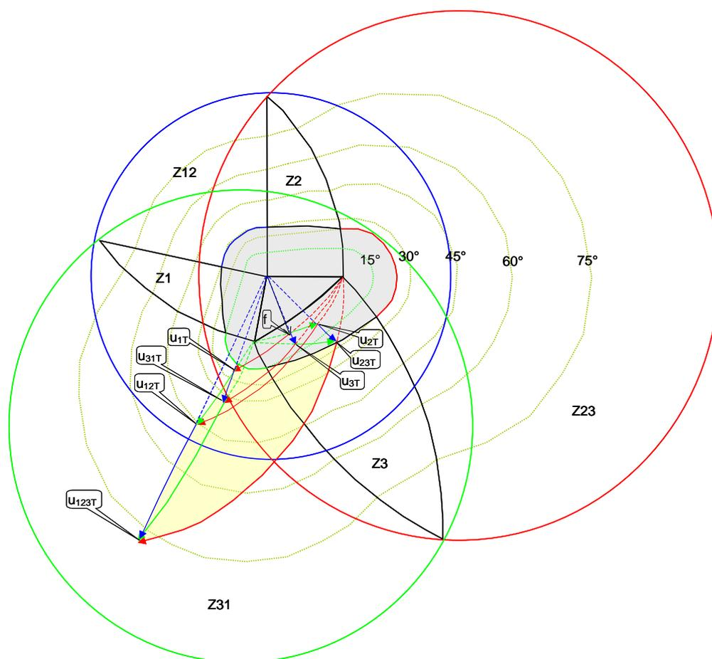
Fig. 8 Completion of plot to define safe (light blue) and danger zone (light yellow) for water pressures superimposed on friction iso-lines kinematics of possible movement.
