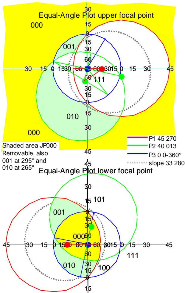
Fig. 3 Plot of great circles P1, P2, P3 and slope on extended equal angle net confirming that the Londe wedge is removable. Inner circle is lower hemisphere and outer area upper hemisphere.
