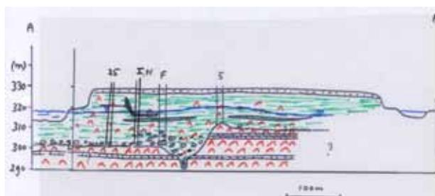
Fig. 9 Cross section along AA' of the map of Figure 8. The black outline shows the location chosen for dam construction.
