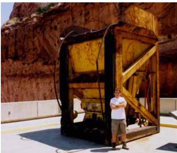
Fig. 3 Bucket which was used to pour concrete (source: author's photo).
