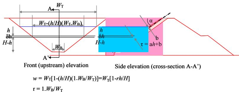
Fig. 1 Model used to solve for overall membrane permeability k.
