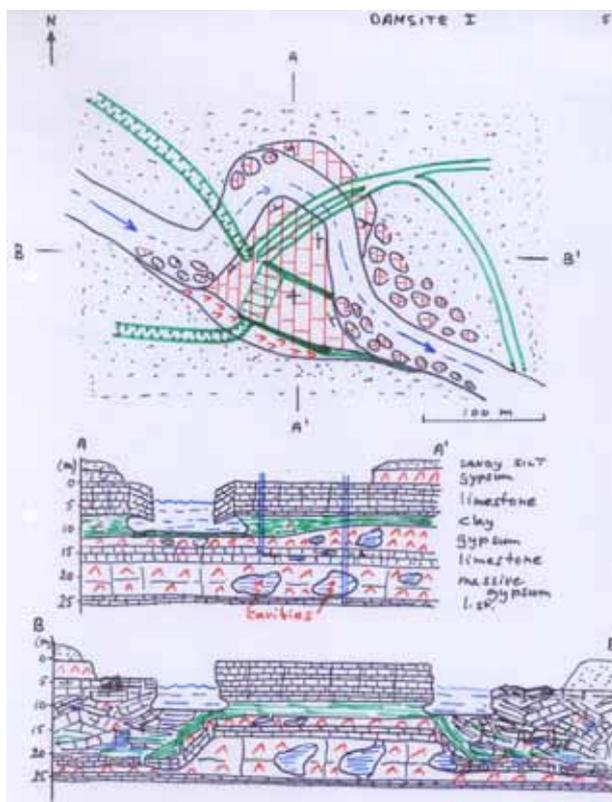
Fig. 6 Sketch of the design of the dam on site I, with cross sections made after the results of the borehole investigation became available.
