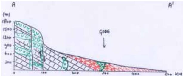
Fig. 3 Section AA' of geological map in Fig. 2. Basement rock is Jurassic limestone overlain by gypsum rock and sandstones, which are invaded by dolerite and basalt related to the African Rift system.
