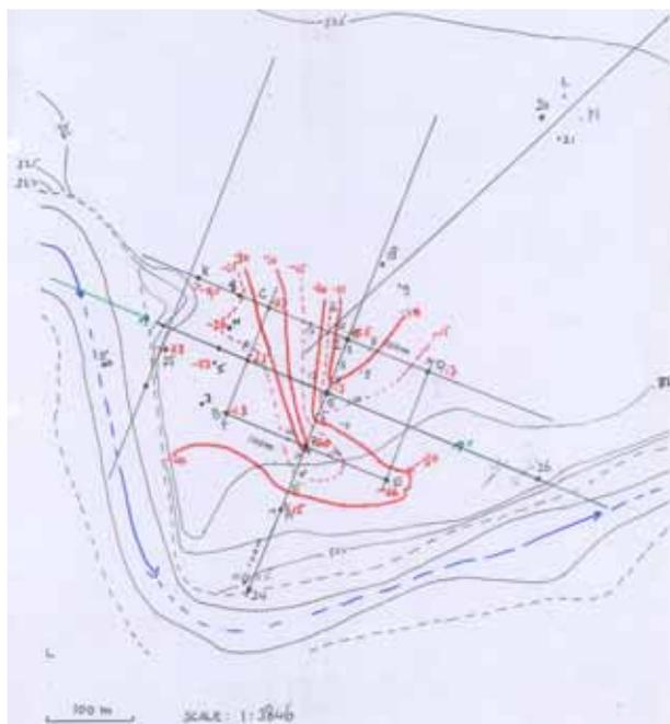
Fig. 8 After the results of the auger drilling through the clay soil became available (red numbers give depth to rock), a depth contour map of gypsum rockhead could be made. This map shows the outline of a steep gorge in the gypsum rock in the subsurface.
