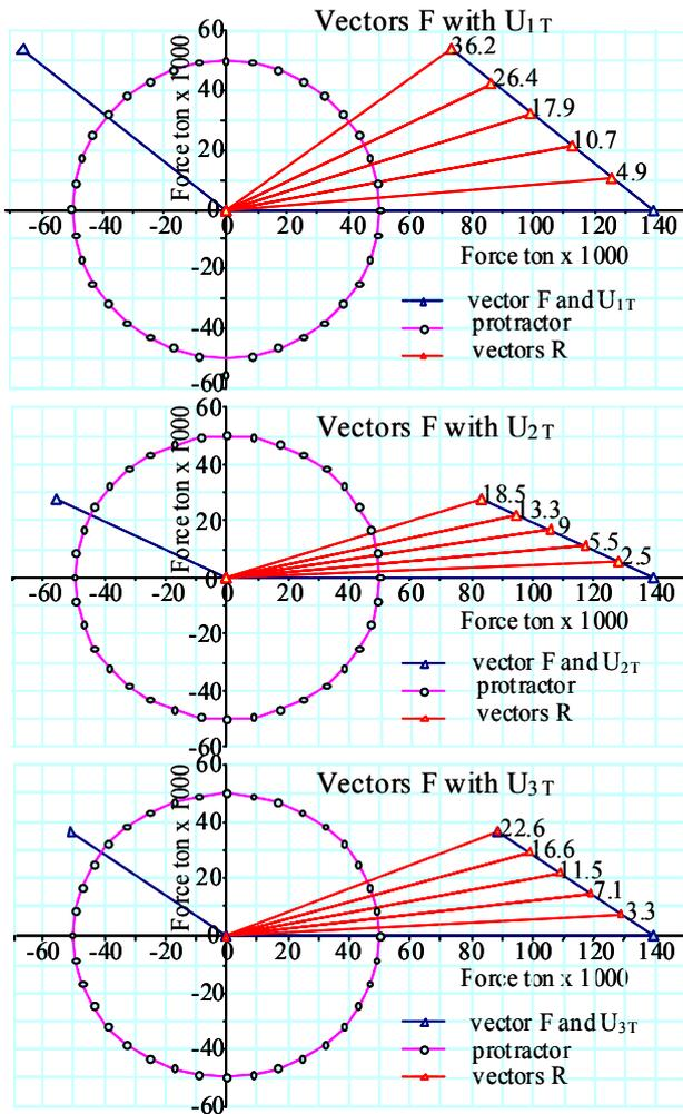
Fig. 6 Influence of water pressure forces on wedge planes P1, P2 and P3 with force F from the dam's weight, weight of the foundation wedge and the hydraulic force of the reservoir. Not surprisingly, plane P1 has the most influence on rotation of the resultant force R (note that rotations are from F in common great circle planes F &  $U_{1T}$ , F &  $U_{2T}$  and F &  $U_{3T}$ . The rotation angles are given in degrees (r values) at the ends of the R vectors.
