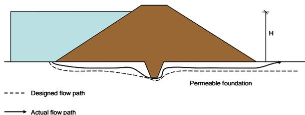
Fig. 2 Schematic representation of seepage under dam foundation causing piping.
