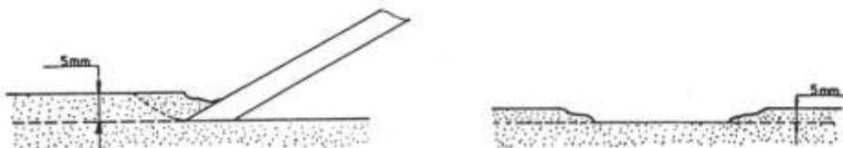
Figure 4. The brittle type of failure.
