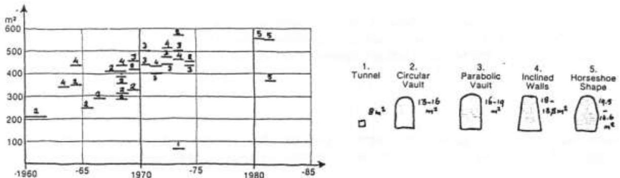
Figure 2 Development of cross-section area of unlined oil storage caverns in Finland between 1960 and 1983.
