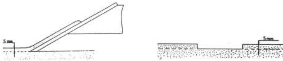
Figure 2. The ductile type of failure.
