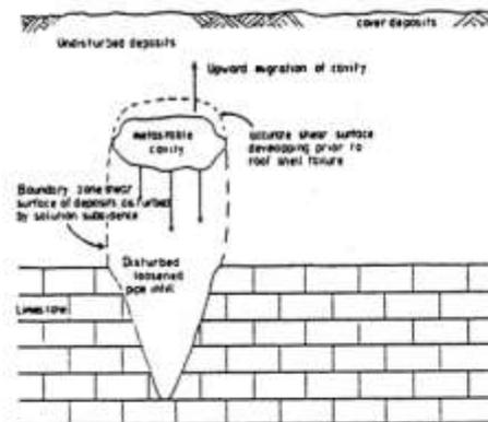
Figure 2 Formation of metastable cavity by solution subsidence
