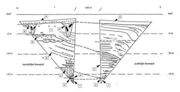
Figure 4 Geological section of the two building pits.
