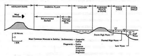
Generalized cross section across a typical coastal Sabkha with typical surface features.
