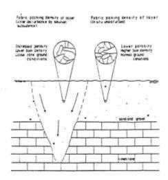
Figure 1 Formation of loose zone ground conditions by solution subsidence.
