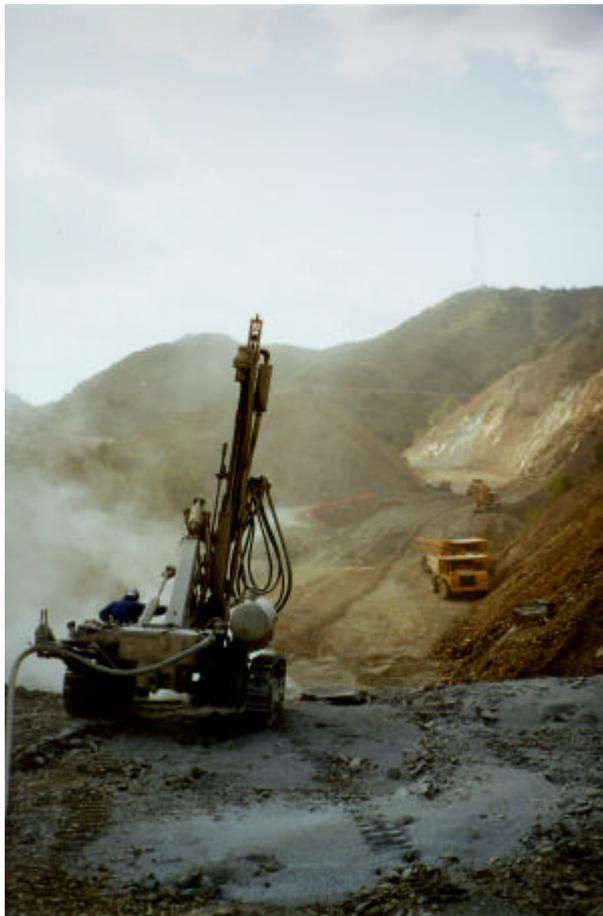
*Figure 4. Drilling blastholes at slope D13; D11 and D12 in the background*
