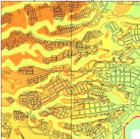
**Figure 7.** *Seismic acceleration response distribution for 2-4 story buildings*
