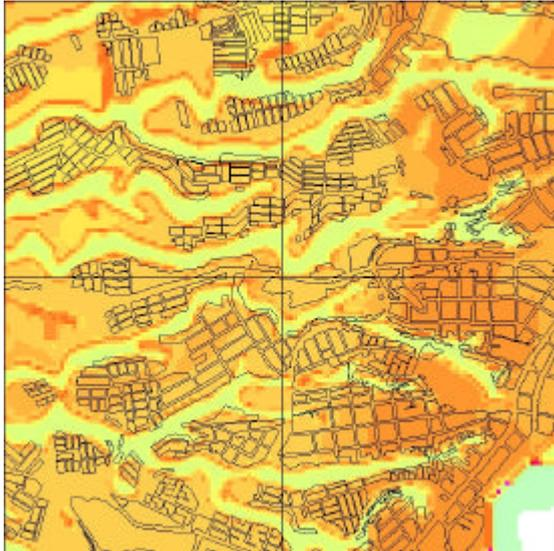
**Figure 6.** *Seismic acceleration response distribution for 1-2 story buildings*
