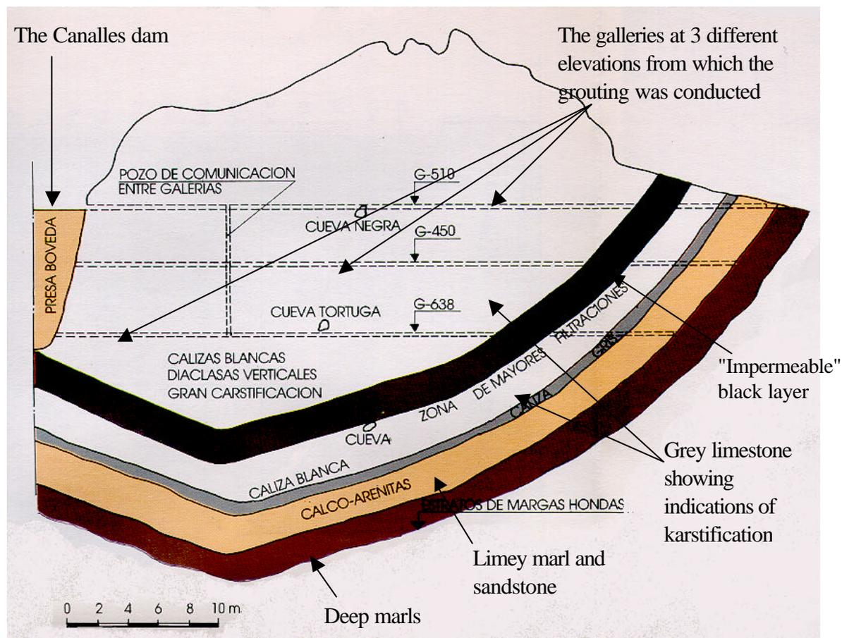
**Figure 2.** A geological section through the left bank of the dam.(source ENHER brochure of the Canalles dam).
