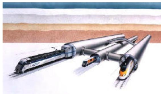
*Figure 3 Three interconnected tubes of Channel Tunnel*
