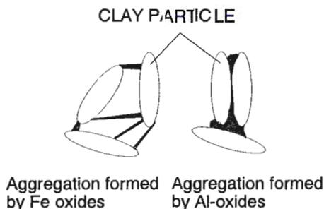
Figure 2 Microstructure Models of Aggregates.
