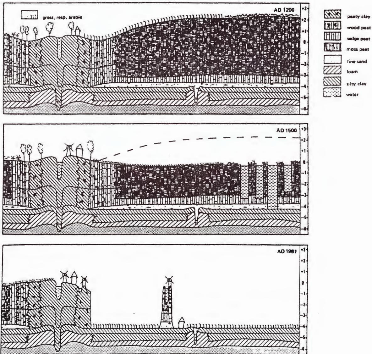
Figure 3 Typical cross-sections through a peat deposit [de Bakker 1988].
