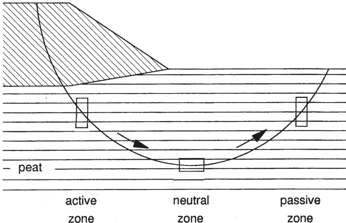
Figure 4 Loading conditions along a potential failure surface.
