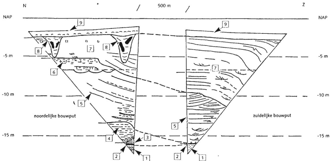
Figure 4 Geological section of the two building pits.
