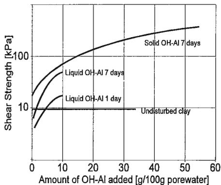
Figure 1 Shear strength in stabilized clay measured by fallcone test as a function of added OH-Al.
