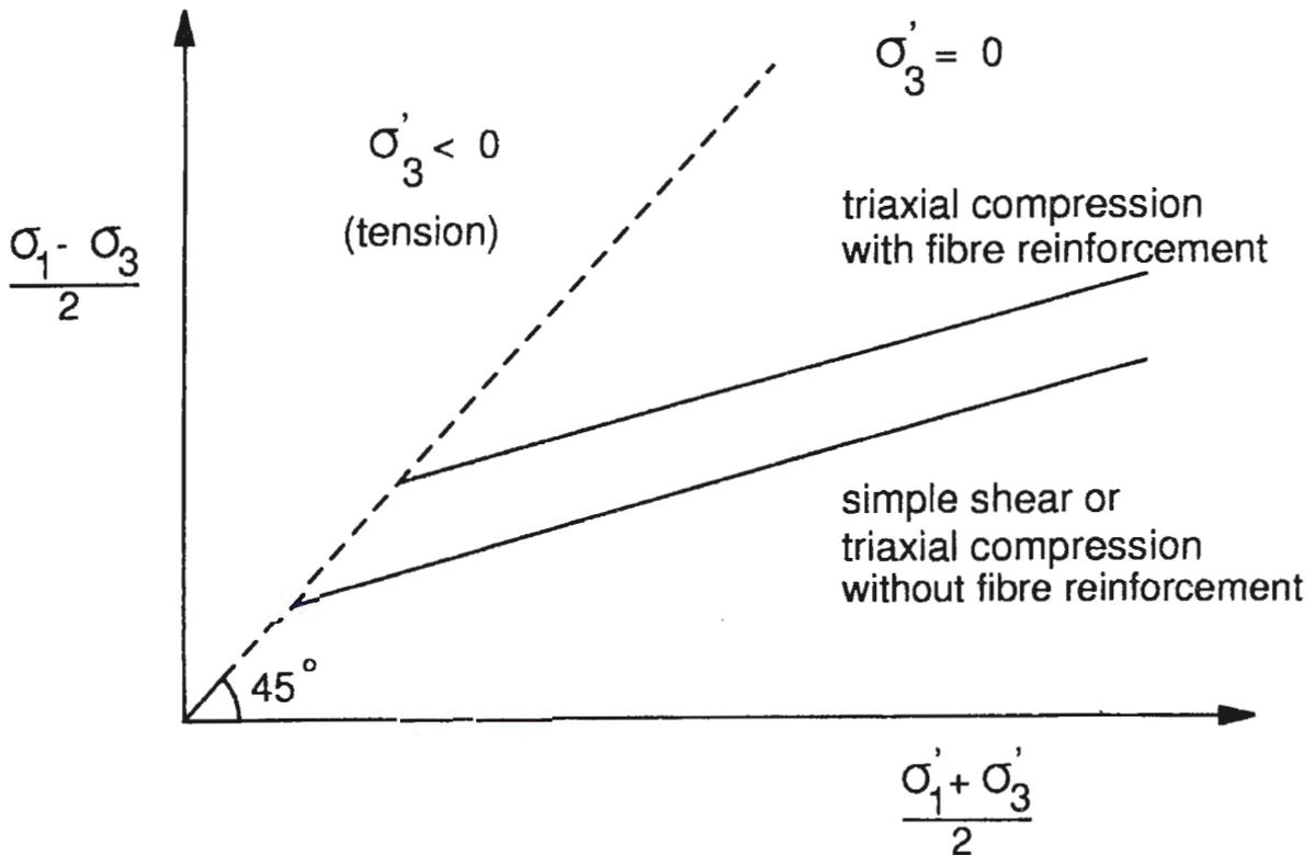
Figure 5 Triaxial compression versus simple shear
