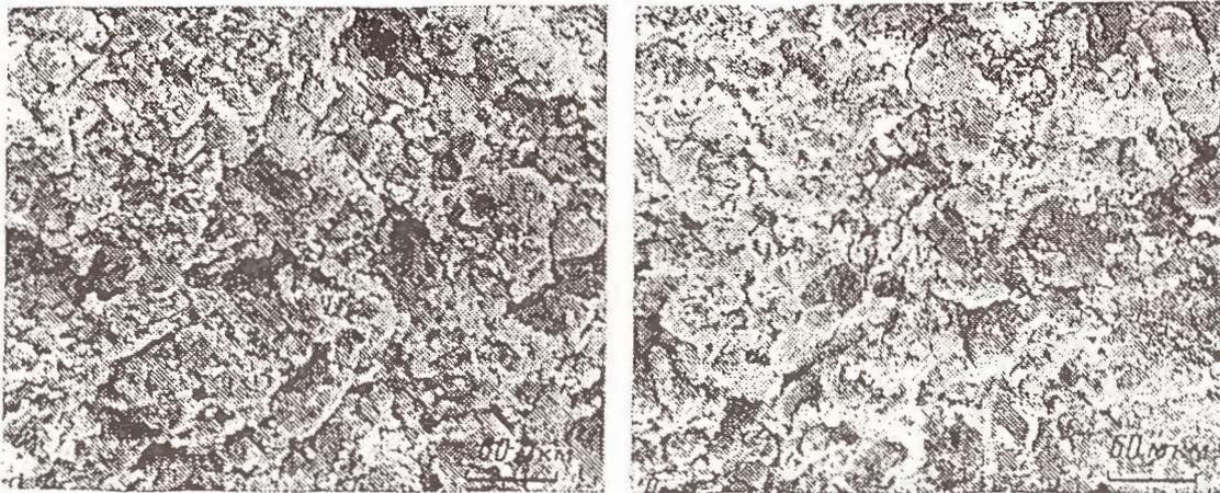
**Figure 11.** Microstructure of undisturbed loess (left) and saturated compacted loess from the impact zone of technogenic element (right) (after Osipov, 1989)
