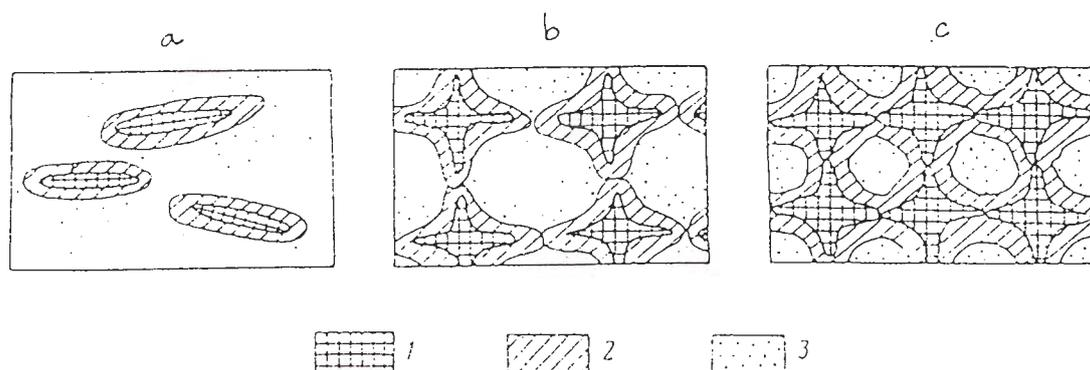
**Figure 1.** Structure types of the middle layer of geotechnogenic massif: a. matrix structure, b. pseudo-completed structure, c. completed structure; 1. technogenic element (inclusion), 2. impact zone of technogenic element, 3. undisturbed soil.
