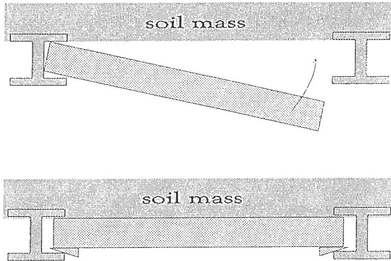
figure 1.3 - support method in Berliner Bauweise
