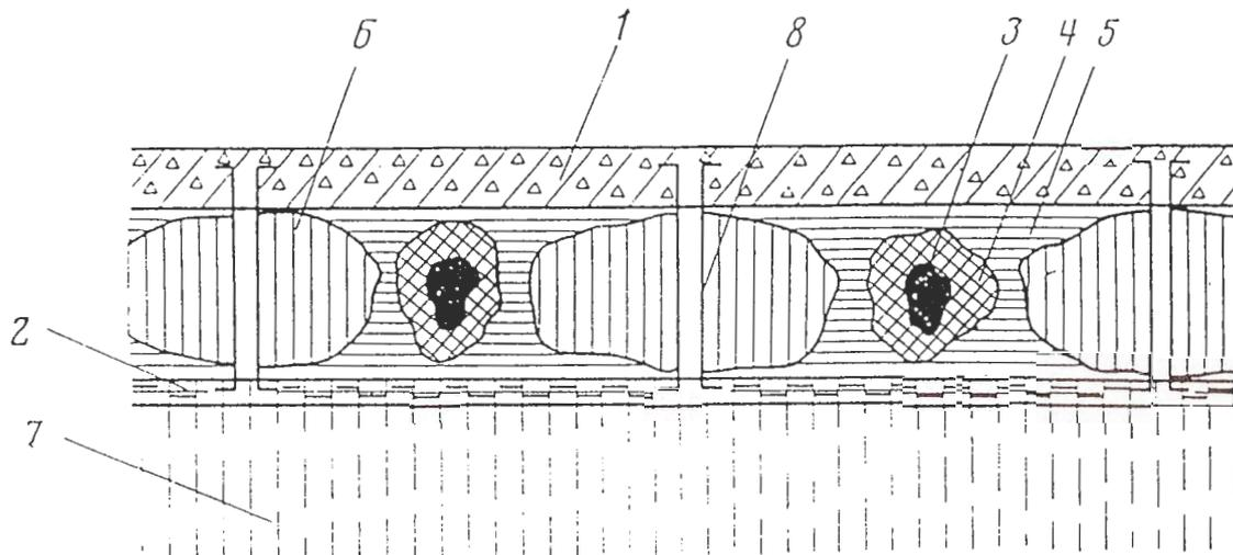
**Figure 13.** Design of the horizontal bearing element of geotechnogenic massif: 1. upper ferroconcrete slab, 2. lower ferroconcrete membrane 3. ground-cement bloc, 4. ground strengthened by penetrating ground-cement mixture, 5. zone of highly compacted ground, 6. zone of normally compacted ground, 7. layer of loess preliminary compacted before construction works, 8. tendons binding upper and lower ferroconcrete slabs.
