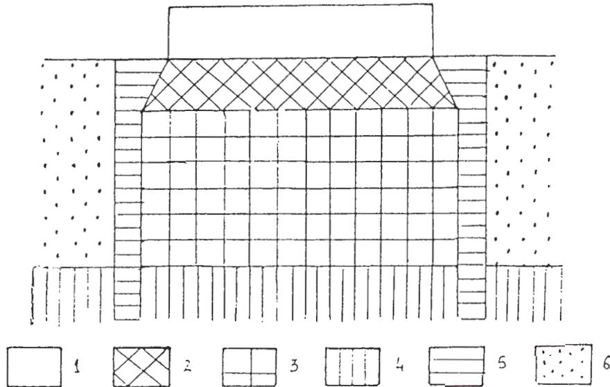
Figure 7. General layout of geotechnogenic massif: 1. Engineering construction, 2. horizontal bearing element, 3. middle layer of improved loess, 4. layer of uncollapsible loess, 5. outline casing, 6. surrounding collapsible loess.
