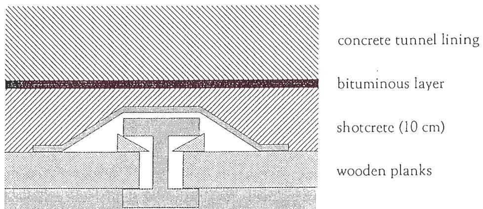
figure 1.4 - construction of tunnel lining
