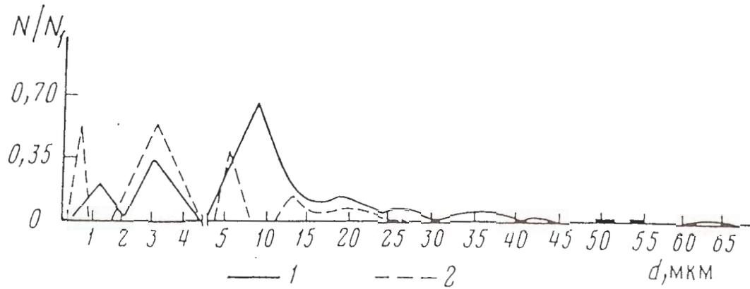
Figure 12. Pore-size distribution plots: 1. undisturbed loess, 2. loess from the impact zone of technogenic element.,  $N/N_1$  probability (after Osipov, 1989)
