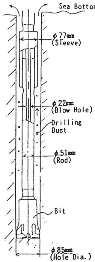
**fig.15:** Drilling a borehole to be filled by demolition agents [Miura, H. et al. (1992) p5].
