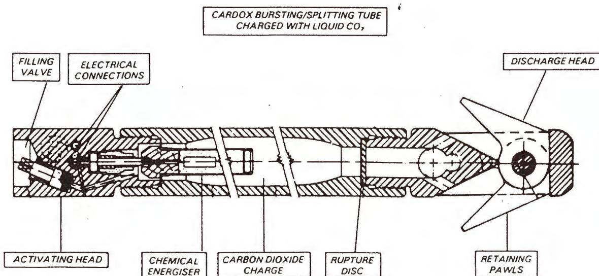
fig.19: The Cardox splitting tube, charged with liquid carbon dioxide [Cardox Company (1992) p3].
