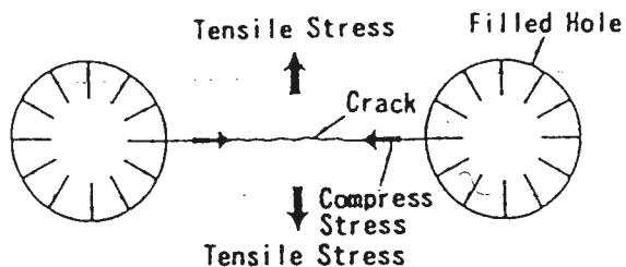
fig.12: Produced cracks, connecting the boreholes, due to generated tensile stresses, [Miura, H. et al. (1992) p3].
