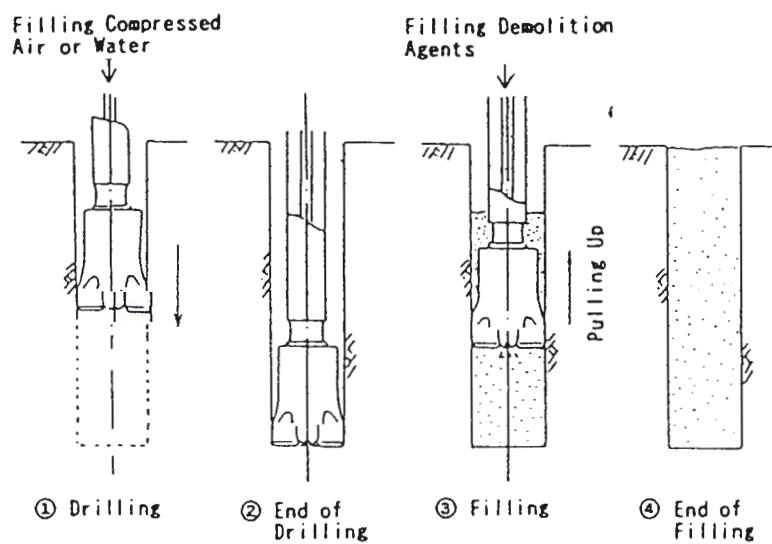
**fig.16:** Filling of the borehole by demolition agents [Miura, H. et al. (1992) p7].
