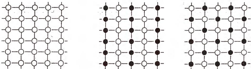
fig.18: Different borehole configurations: respectively empty boreholes alone, a combination of empty and filled boreholes in a parallel way and a combination of empty and filled boreholes in a zigzag arrangement [Miura, H. et al. (1992) p7].
