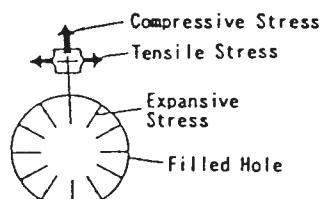
**fig.10:** Development of compressive and tensile stresses [Miura, H. et al. (1992) p3].
