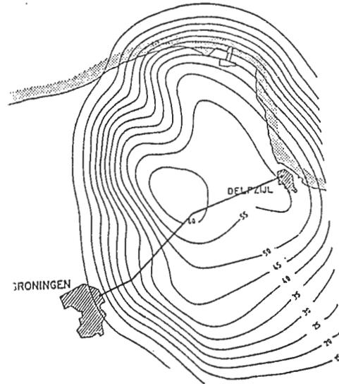
Figure 2 isolines of subsidence. (N.A.M.)
