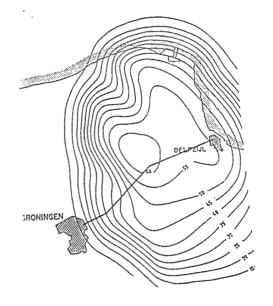
Figure 2 isolines of subsidence. (N.A.M.)
