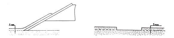
Figure 2. The ductile type of failure.
