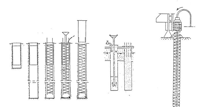
Figure 2: Construction of a bored pile.
