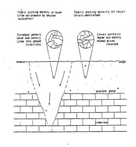
Figure 1 Formation of loose conditions by zone ground
