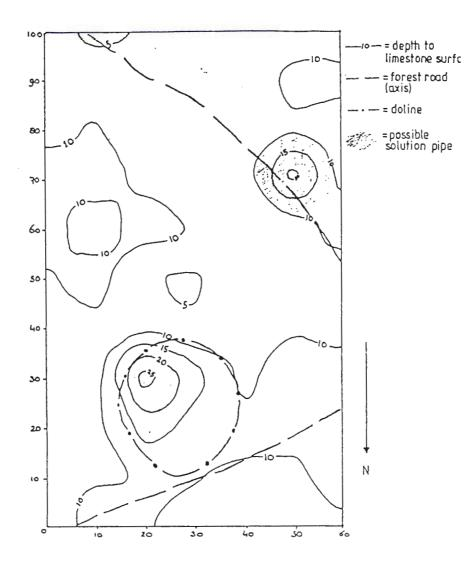
Figure 5 Contourmap of the depth to the limestone
