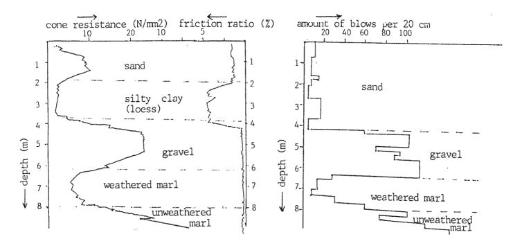
Figure 1: Typical results of cone penetration test and heavy penetration test (schwere rammsondierung).
