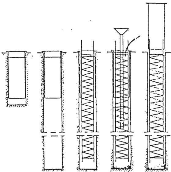
Figure 2: Construction of a bored pile.
