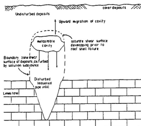
Figure 2 Formation of metastable cavity by solution subsidence
