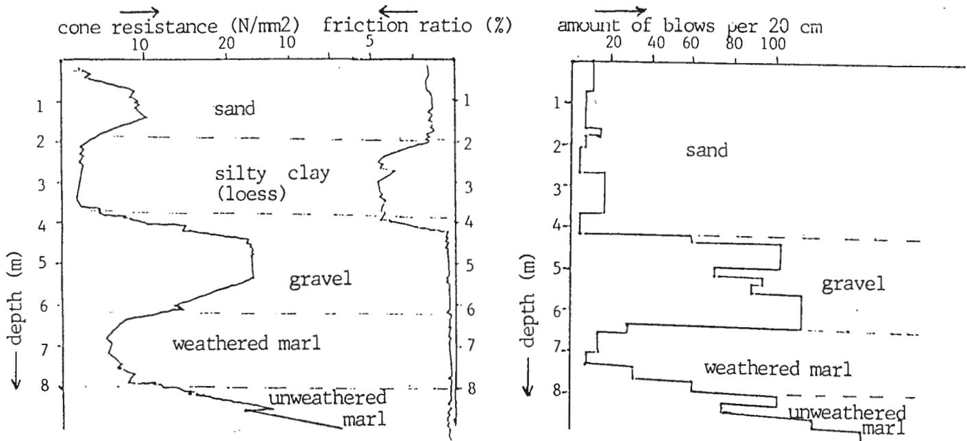
Figure 1: Typical results of cone penetration test and heavy penetration test (schwere rammsondierung).
