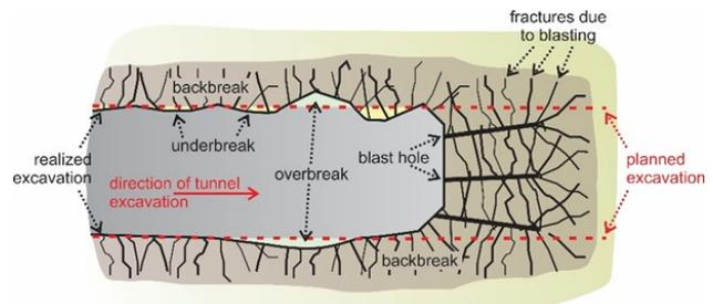
Figure 3 Discontinuities in a groundmass due to blasting and present as backbreak in the walls, roof, and floor of a tunnel give access for weathering agents
