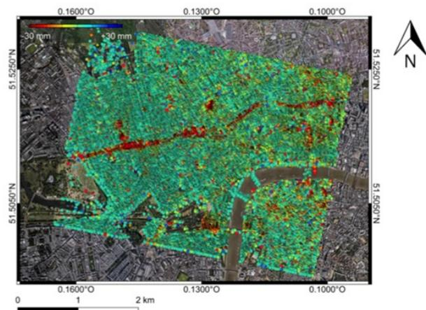
*Figure 1 Example of satellite-based map of ground movement: Crossrail tunnel excavation in London, UK.*
