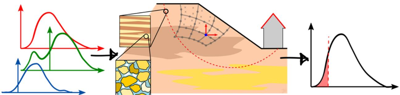
*Figure 1: Uncertainty propagation in stochastic modelling of geotechnical stability as the basis for reliability-based assessment.*
