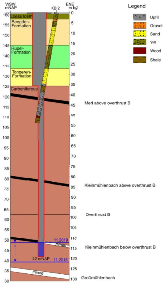
Figure 4 Cross-section through shaft DOM 37. The mine water has recently invaded the bottom of the shaft.
