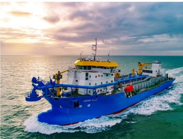
Figure 1 NMDC's Trailing Suction Hopper Dredger "Arzana"
