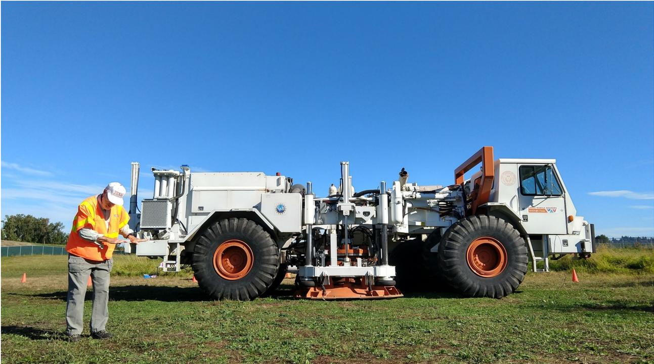
Figure 3 Professor Ken Stokoe from University of Texas, Austin, explaining how the big shaker T-Rex induced shear waves to induce small earthquakes and test the potential of bio-based treatment for liquefaction mitigation in Portland, Oregon.
