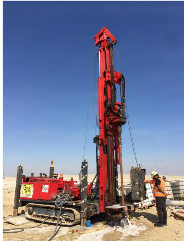
*Drilling machine for rock cores in the upper sections of the Eocene Rus formation, up to a depth of 150m .*
