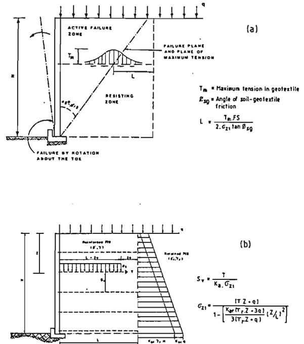
Figure 6. Design criteria for reinforced soil walls. (From ref. 12). (a) Rankine failure surface and calculation of reinforcement anchor length. (b) Vertical stresses behind reinforced soil wall and calculation of reinforcement spacing.
