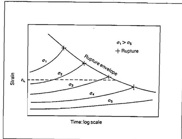
Figure 2. Generalised creep curves for geotextiles. (From ref. 9)
