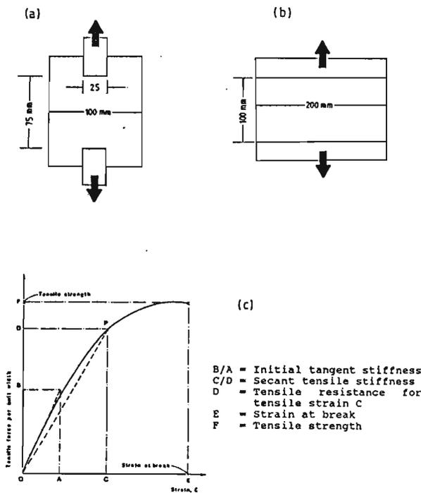
Figure 1. Tension tests for geotextiles. (a) Grab method (ASTM D-1682, DIN 53858). (b) Wide strip method (ASTM D-4595). (c) Typical tensile force per unit width-strain curve.
