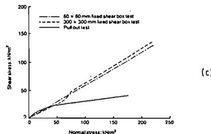
Figure 3. Measurement of reinforcement-soil interaction characteristics: (a) Direct shear test. (b) Pullout test. (c) Typical results (heatbonded non-woven geotextile). (From ref. 9)
