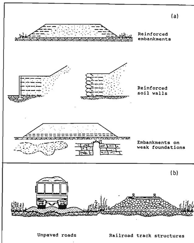
Figure 4. Types of reinforced soil structures. (a) Earth structures. (b) Load-supporting structures. (From ref. 12).
