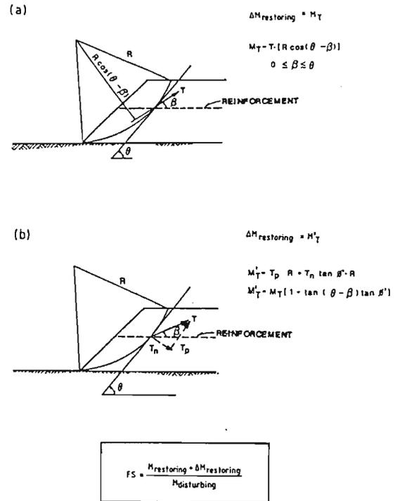
Figure 5. Design criteria for reinforced slopes. (From ref. 12) (a) Reinforcement force assumed to act as independent force. (b) Reinforcement force assumed to increase soil strength.
