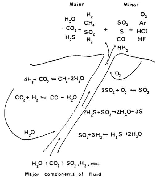
Figure I. Some chemical reactions in a fumarolic conduit. (Lyon, G.L., 1974)
